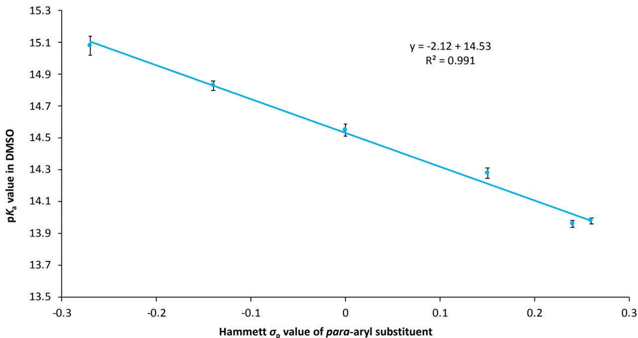
**Figure S1.** The correlation between the  $pK_a$  values of the triazolium salts **12** in DMSO at 25 °C and the Hammett  $\sigma_p$  value of the 4-aryl substituent.<sup>35</sup> The original data is reproduced from Cheng *et al.*<sup>34</sup>
