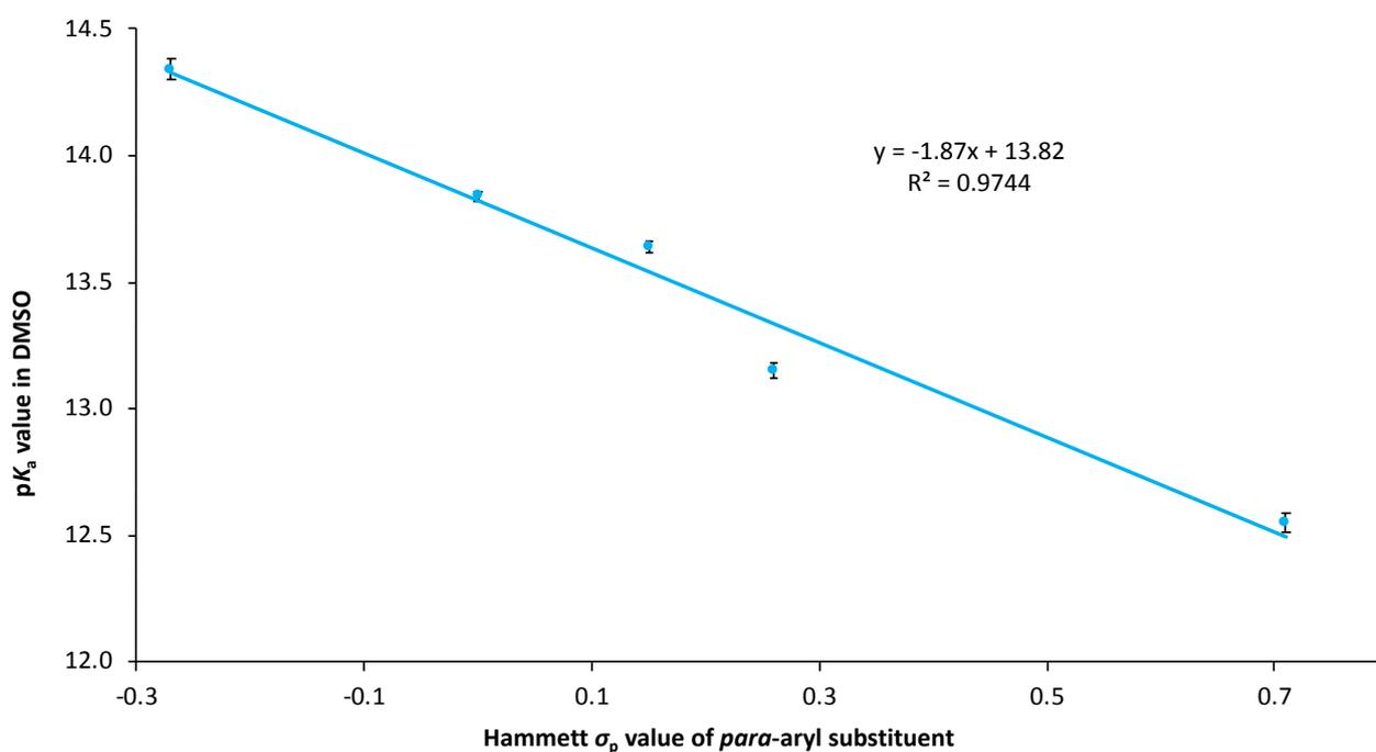
**Figure S2.** The correlation between the  $pK_a$  values of the triazolium salts **13** in DMSO at 25 °C and the Hammett  $\sigma_p$  value of the 4-aryl substituent.<sup>35</sup> The original data is reproduced from Cheng *et al.*<sup>34</sup>
