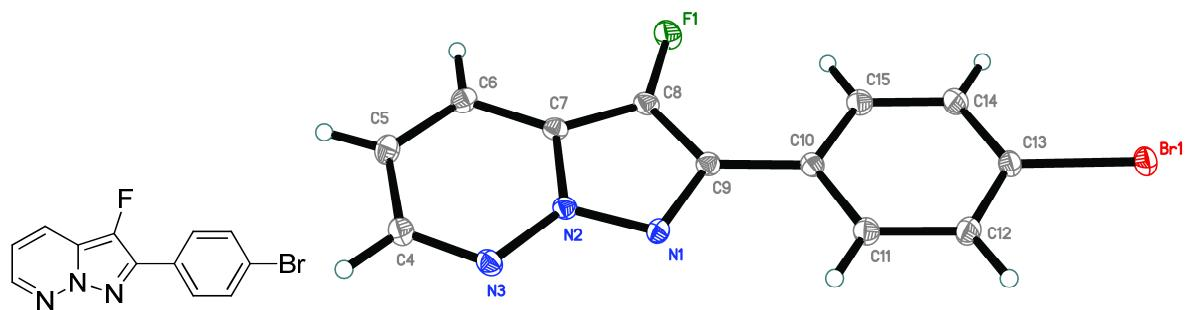
General view of the compound **10c** in representation of atoms *via* thermal ellipsoids at 50% probability level.
