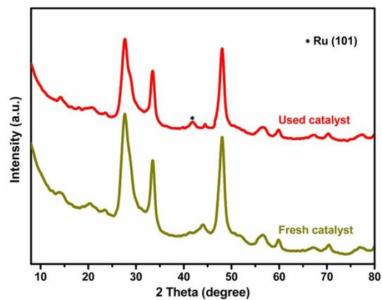
**Figure S1.** PXRD patterns of the synthesized ternary ZIS-CN-G nanocomposite before and after photocatalytic experiments.
