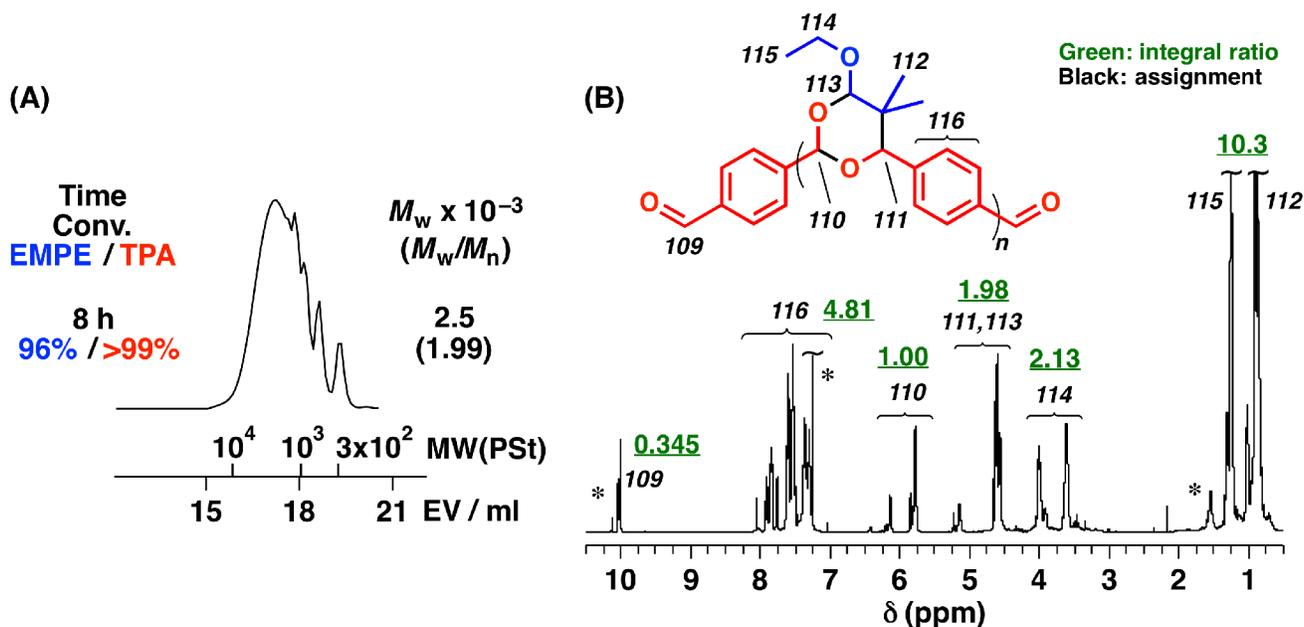
**Figure S8.** (A) MWD curve and (B)  $^1\text{H}$  NMR spectrum of the product obtained by the polyaddition of EMPE and TPA ( $[\text{TPA}]_0 = 0.50$  M,  $[\text{EMPE}]_0 = 0.50$  M,  $[\text{EtAlCl}_2]_0 = 50$  mM,  $[\text{THF}] = 1.0$  M, in dichloromethane at  $0^\circ\text{C}$ ; \* solvent, residual monomer, or water; number written in green: integral ratio).
