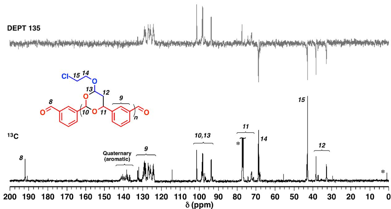
**Figure S4.** <sup>13</sup>C and DEPT 135 NMR spectra of the product obtained by the copolymerization of CEVE and IPA (in CDCl<sub>3</sub> at 30 °C; [TPA]<sub>0</sub> = 0.50 M, [CEVE]<sub>0</sub> = 0.50 M, [EtAlCl<sub>2</sub>]<sub>0</sub> = 50 mM, [THF] = 1.0 M, in dichloromethane at 0 °C; a different sample from those shown in Figures 2 and 3; reprecipitated from methanol; \* solvents or grease).
