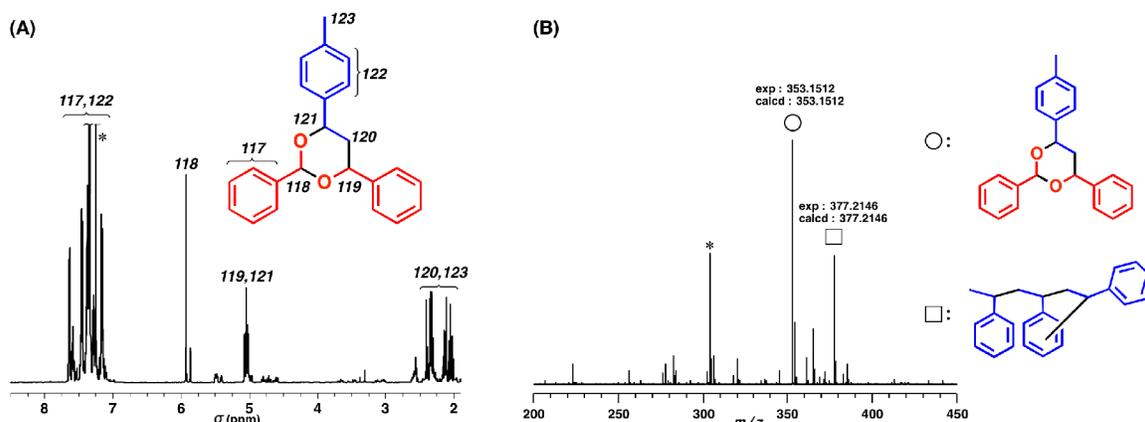
**Figure S10.** (A)  $^1\text{H}$  NMR (in  $\text{CDCl}_3$  at  $30\text{ }^\circ\text{C}$ ; \*  $\text{CHCl}_3$ ) and (B) ESI-MS spectra of the low-molecular-weight portion of the product obtained by the reaction of pMeSt and BzA (the low-molecular-weight portion of the sample shown in Figure S9).
