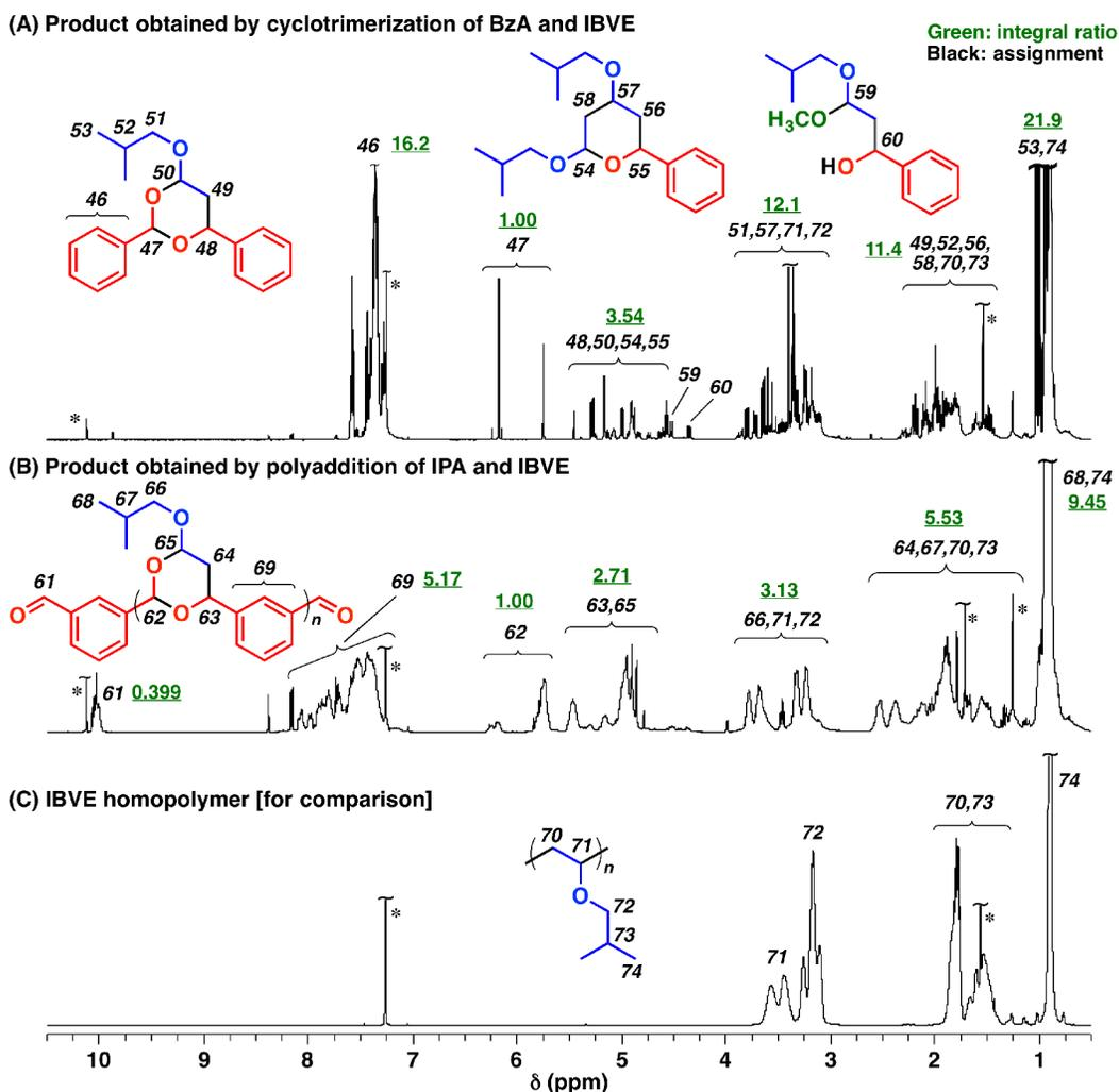
**Figure S2.** <sup>1</sup>H NMR spectra of (A) the product obtained by the cyclotrimerization of BzA and IBVE (entry 2 in Table 1), (B) the product obtained by polymerization of IPA and IBVE (entry 3 in Table 2), and (C) IBVE homopolymer (\* solvent, residual monomer, water, etc.; number written in green: integral ratio).
