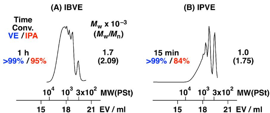
**Figure S5.** MWD curves of the products obtained by the polymerization of IPA with (A) IBVE (entry 3 in Table 2) or (B) IPVE (entry 4).
