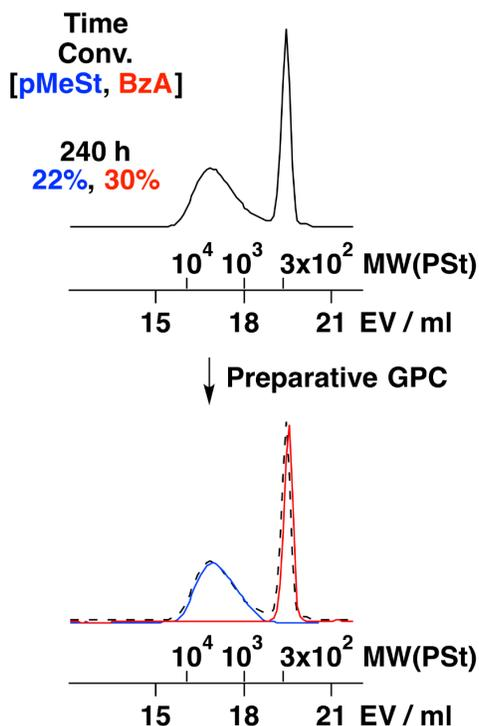
**Figure S9.** MWD curves of the product obtained by the reaction of pMeSt and BzA (upper) and the high- (blue) and low- (red) molecular-weight portions (lower) separated by preparative GPC ( $[\text{pMeSt}]_0 = 0.20$  M,  $[\text{BzA}]_0 = 0.20$  M,  $[\text{GaCl}_3]_0 = 5.0$  mM,  $[\text{DTBP}] = 1.8$  mM, in toluene at  $0^\circ\text{C}$ ).
