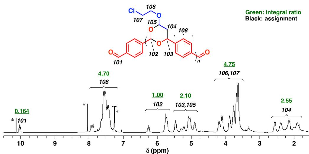
**Figure S7.**  $^1\text{H}$  NMR spectrum of the polymer obtained by the polyaddition of CEVE and TPA (the bottom curve in Figure S6C; \* solvent or residual monomer; number written in green: integral ratio).
