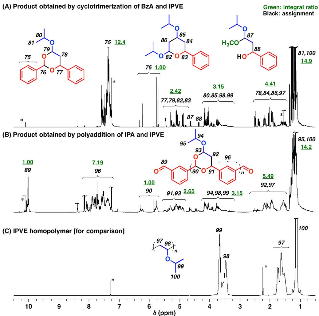
**Figure S3.**  $^1\text{H}$  NMR spectra of (A) the product obtained by the cyclotrimerization of BzA and IPVE (entry 3 in Table 1), (B) the product obtained by polymerization of IPA and IPVE (entry 4 in Table 2), and (C) IPVE homopolymer (\* solvent, residual monomer, or water; number written in green: integral ratio).
