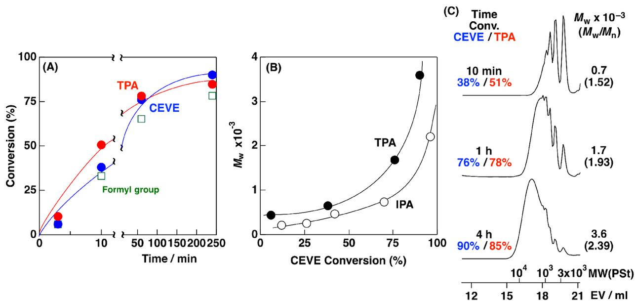
**Figure S6.** (A) Time–conversion curves of polyaddition of CEVE and TPA, (B)  $M_w$  values (the values for IPA are the same to those shown in Figure 3B), and (C) MWD curves of the products obtained (entry 2 in Table 2;  $[\text{TPA}]_0 = 0.50 \text{ M}$ ,  $[\text{CEVE}]_0 = 0.50 \text{ M}$ ,  $[\text{EtAlCl}_2]_0 = 50 \text{ mM}$ ,  $[\text{THF}] = 1.0 \text{ M}$ , in dichloromethane at  $0^\circ\text{C}$ ).
