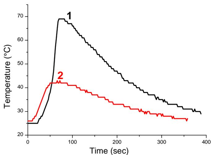
**Figure S6: Redox polymerization:** Optical pyrometric measurements (Temperature vs. mixing time, 4 mm samples), in air in the model methacrylate resin for 2.0 wt% APS (+2.0 wt% water) mixed 1.5 wt% 2dppba and with **(1)** 0.3 wt% Fe and **(2)** 1.3 wt% Fe.
