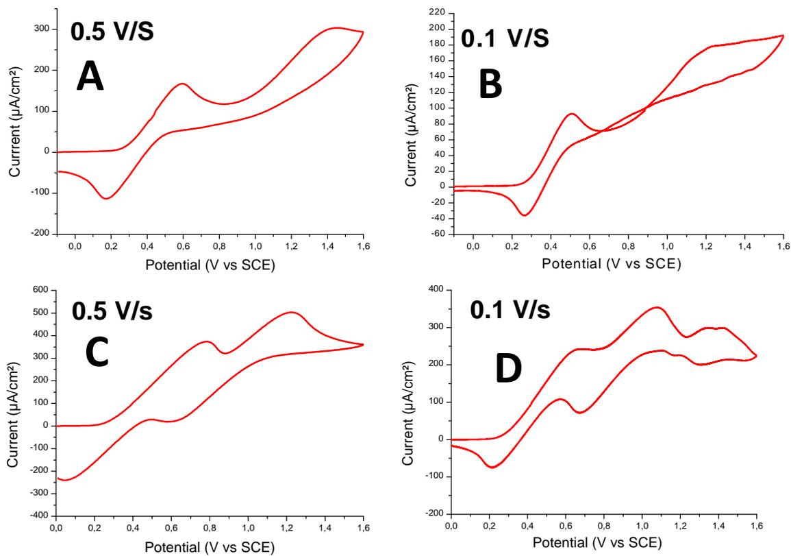
**Figure S7:** Cyclic voltammetry (CV) experiments in ACN (containing 0.2 M tetrabutylammonium hexafluorophosphate,  $\text{N}_2$  degassed)) for **A,B** : Fe + 2dppba and **C,D** Fe + amine (4-N,N TMA).
