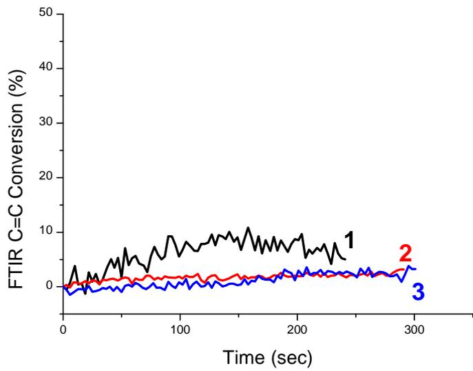
**Figure S5:** Photopolymerization profiles (methacrylate C=C function conversion vs. irradiation time) measured in RT-FTIR for the resin 2; 1.4 mm thick samples, in air for 2.0 wt% Iod and 0.5 wt% Fe(II)
