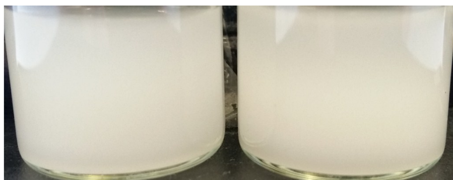
Fig. S15. Formation of a stable emulsion of ethyl acetate/water mixture (3:1) upon addition of PPO 47 - b -PDEGAO 6 (left) and PPO 47 - b -PiGAO 6 (right).
