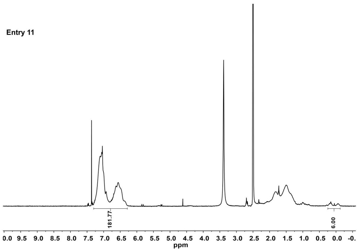
**Figure S28.** <sup>1</sup>H NMR spectrum of **2-PS** in chloroform-*d* at 298 K, related to entry 11, **Figure S19**.
