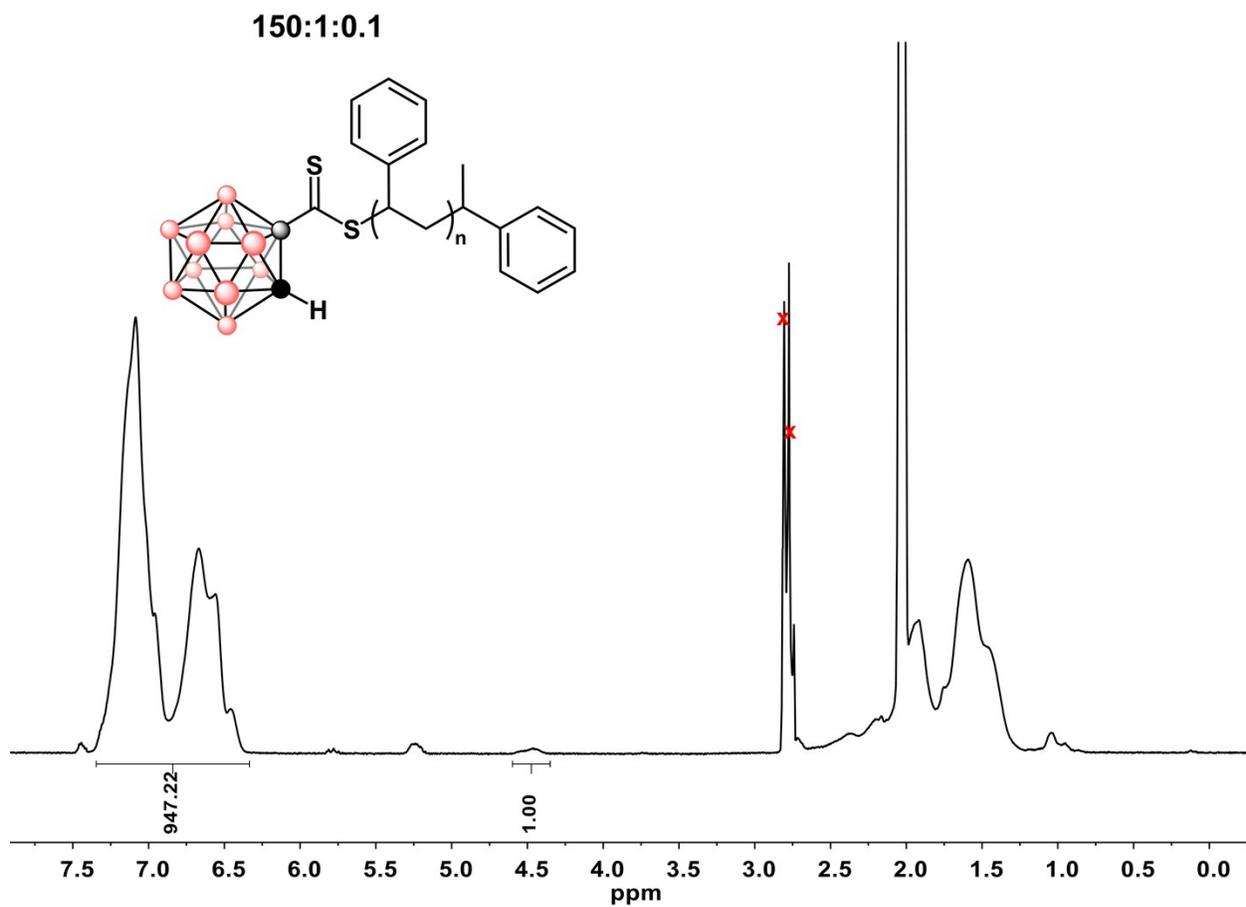
**Figure S13.**  $^1\text{H}$  NMR spectrum of 1-PS in acetonitrile- $d_3$  at 298 K and sample calculation of polymer molecular weight.
