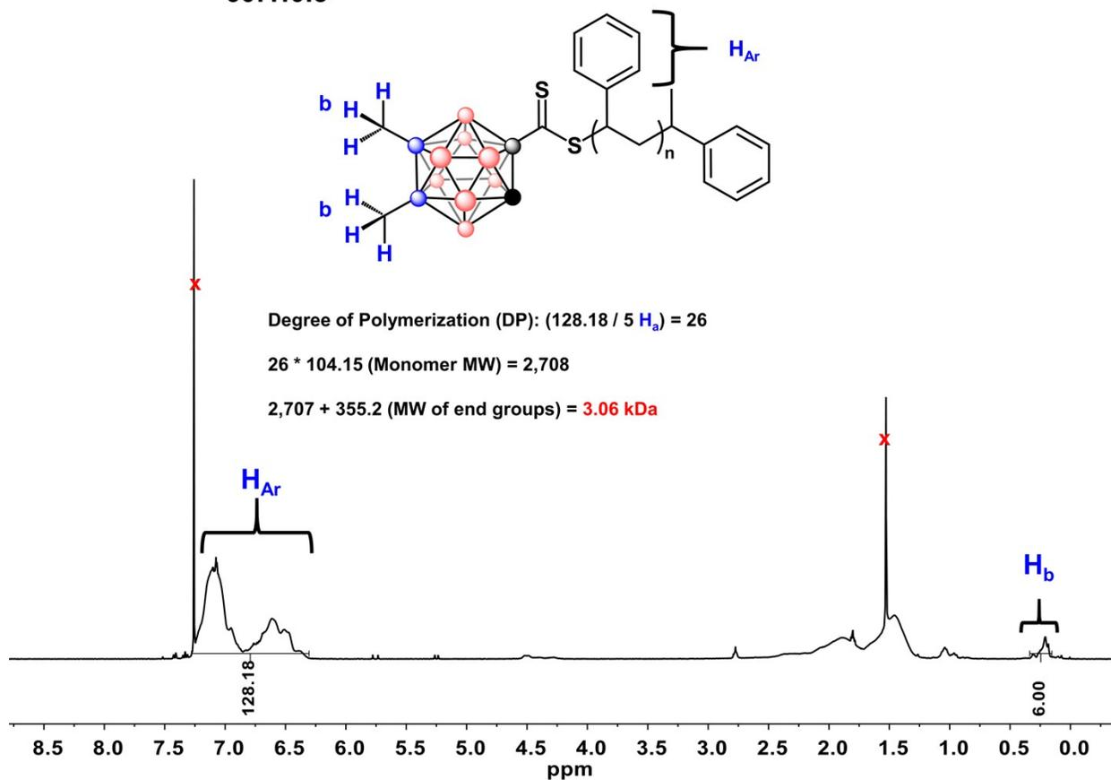
**Figure S14.** <sup>1</sup>H NMR spectrum of 2-PS in chloroform-*d* at 298 K and sample calculation of polymer molecular weight.
