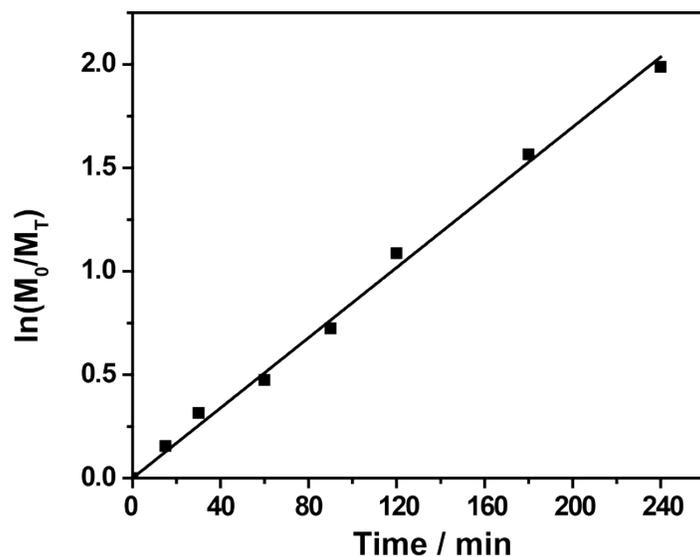
**Figure S34.** Polymer kinetic plot of polymerization of a 2M solution of methyl acrylate in PhMe ( $R^2 = 0.99$ ).
