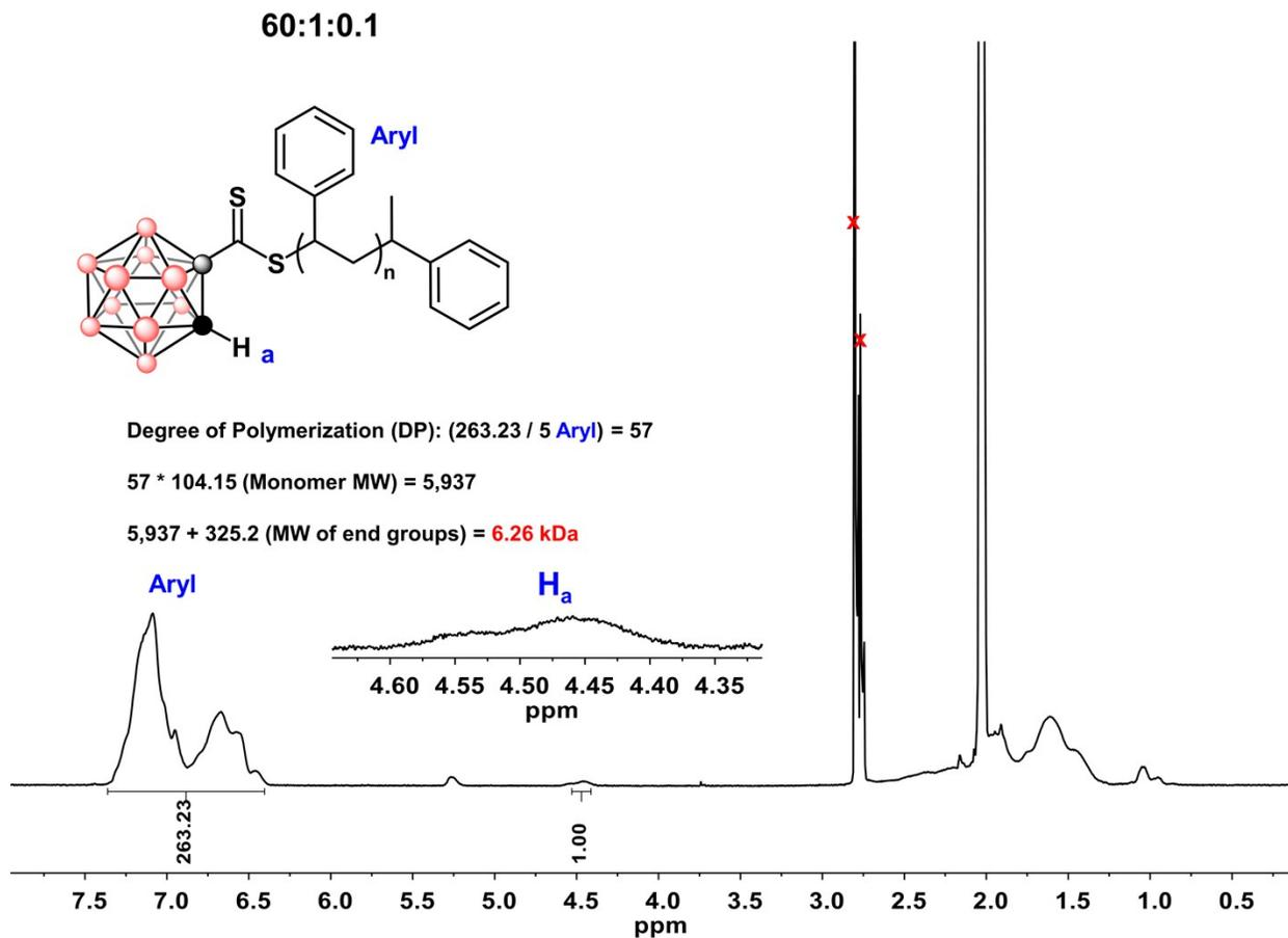
**Figure S12.**  $^1\text{H}$  NMR spectrum of **1-PS** in acetonitrile- $d_3$  at 298 K and sample calculation of polymer molecular weight.
