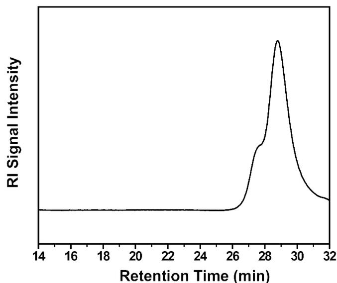
**Figure S36.** GPC spectrum of carborane deprotection reaction, which shows a high degree of polymer coupling over the course of the reaction. GPC acquired using DMF with 0.1 M LiBr as the eluent.
