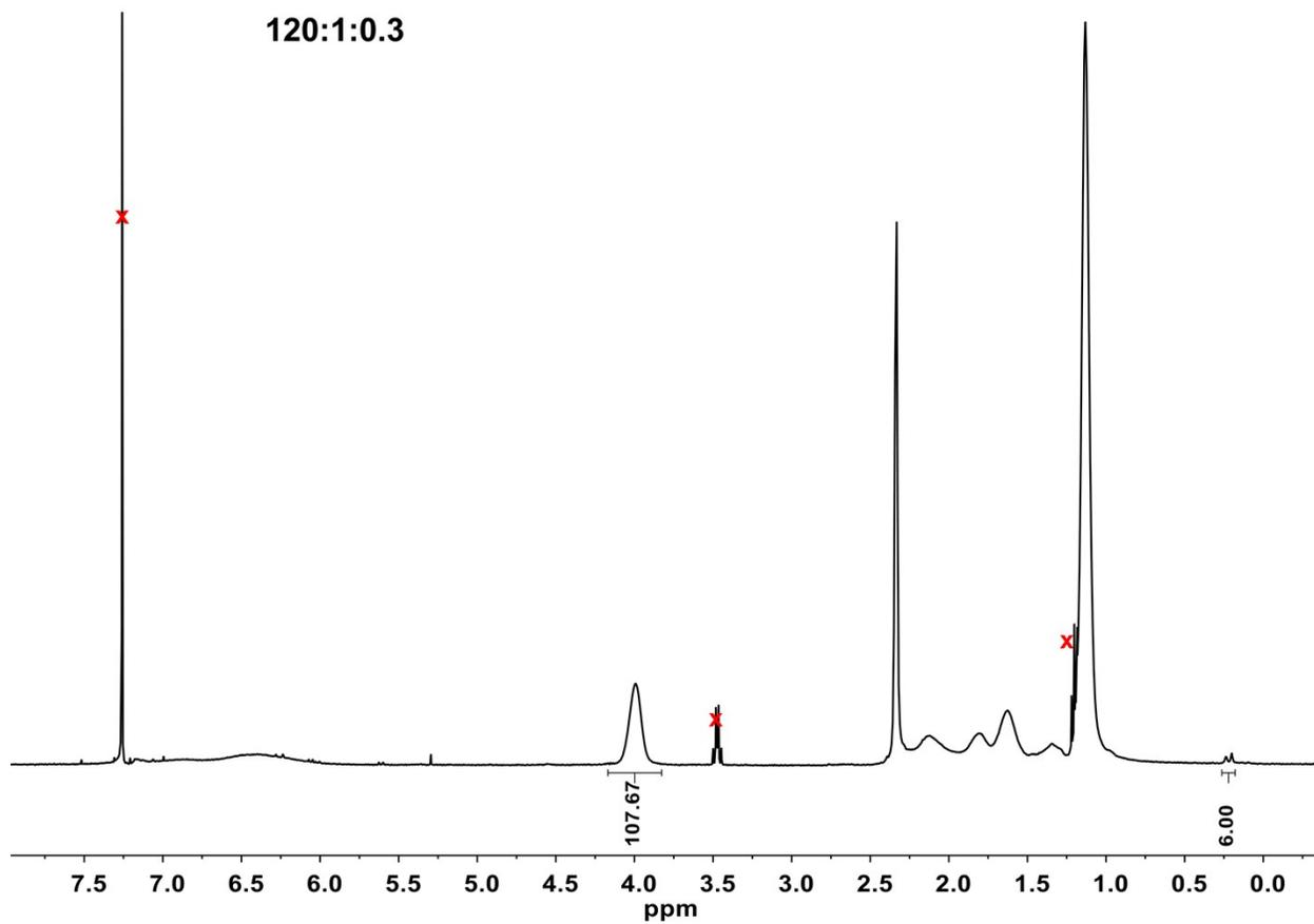
**Figure S17.**  $^1\text{H}$  NMR spectrum of 2-pNIPAAm in chloroform-*d* at 298 K.
