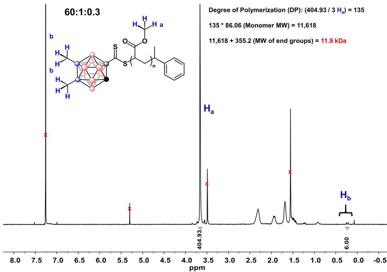
**Figure S22.**  $^1\text{H}$  NMR spectrum of 2-PMA in chloroform-*d* at 298 K and sample calculation of polymer molecular weight.
