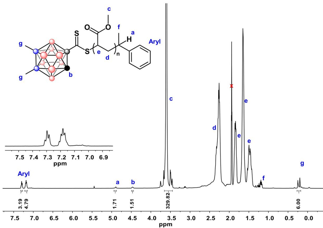
Figure S25.  $^1\text{H}$  NMR spectrum of 2-PMA in acetonitrile- $d_3$  at 298 K.
