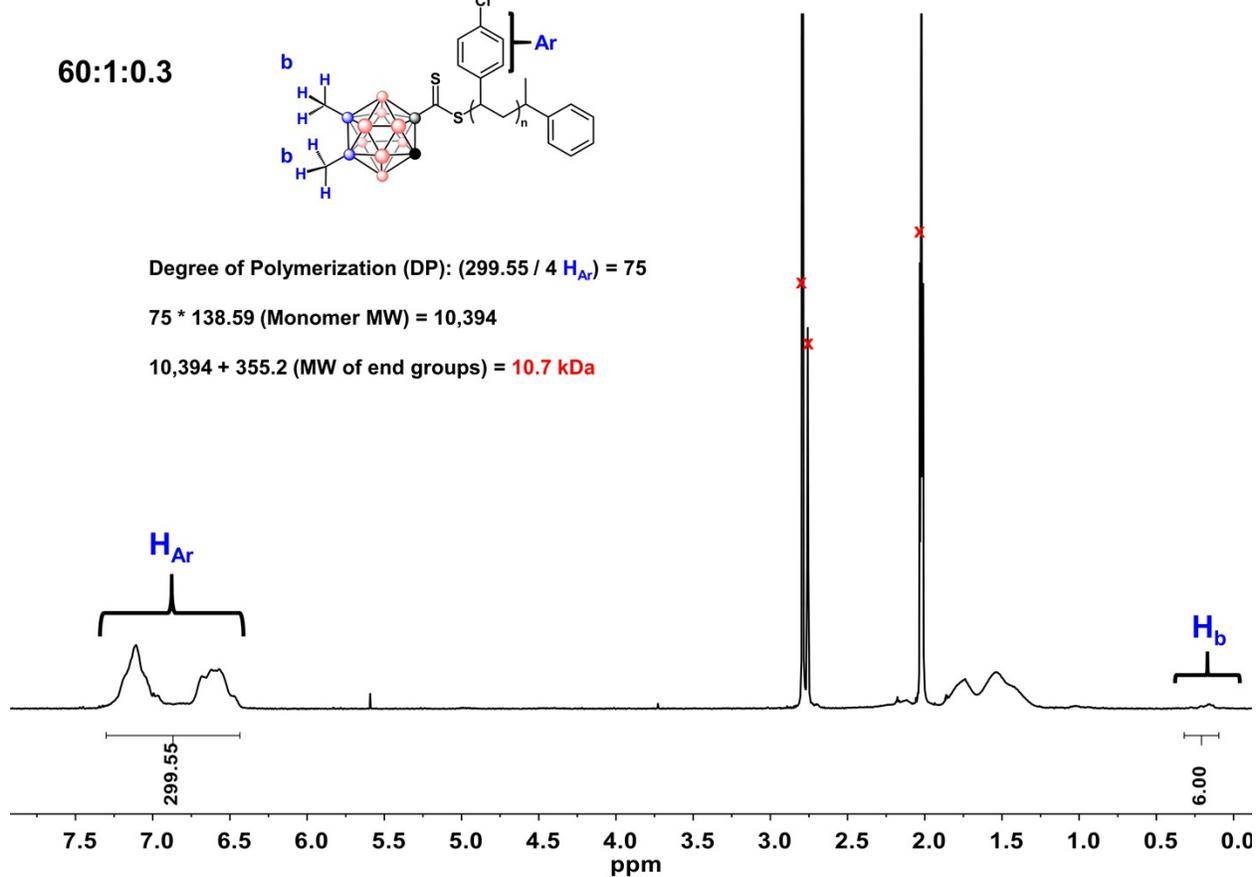
**Figure S19.**  $^1\text{H}$  NMR spectrum of 2-(4-Cl)-PS in acetone- $d_6$  at 298 K and sample calculation of polymer molecular weight.
