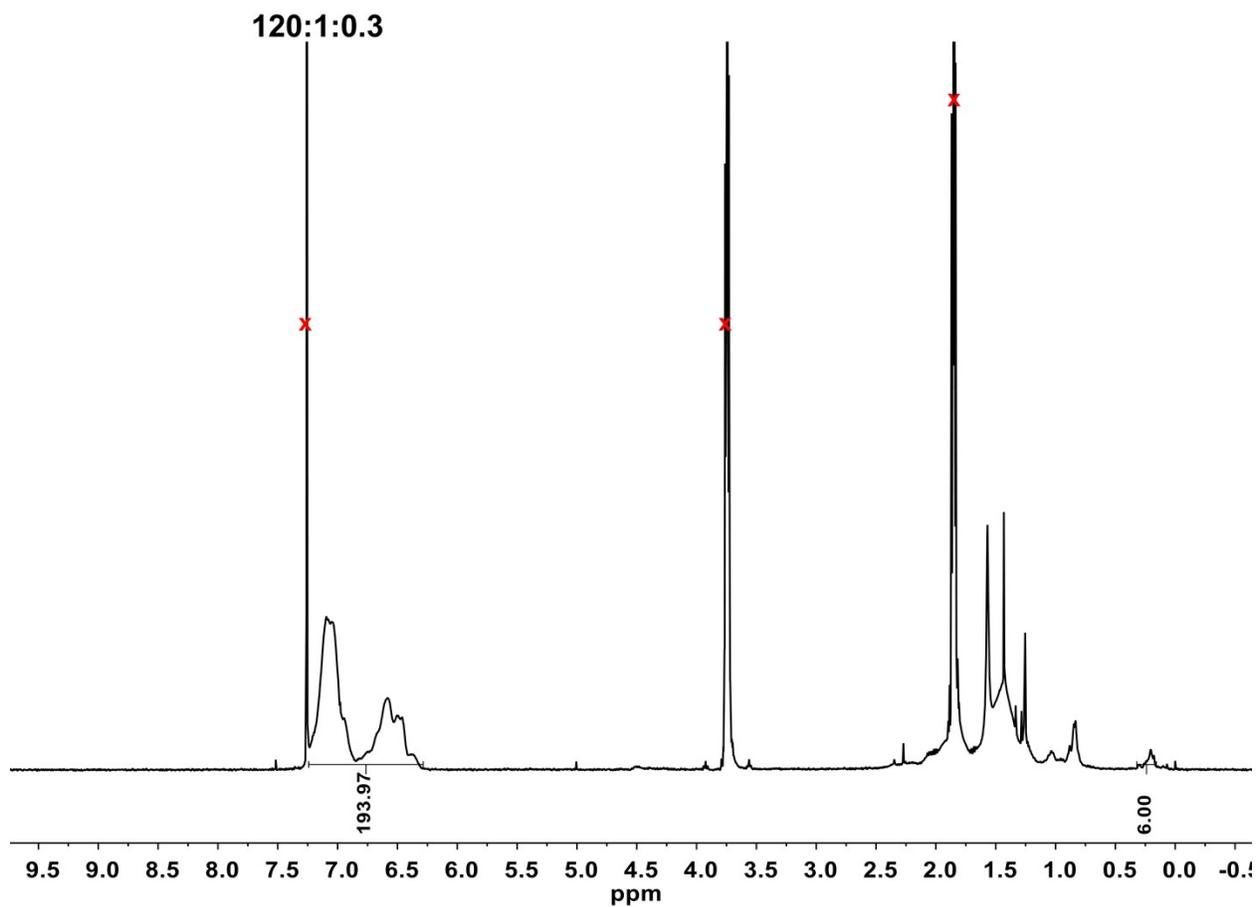
**Figure S15.**  $^1\text{H}$  NMR spectrum of **2-PS** in chloroform-*d* at 298 K.
