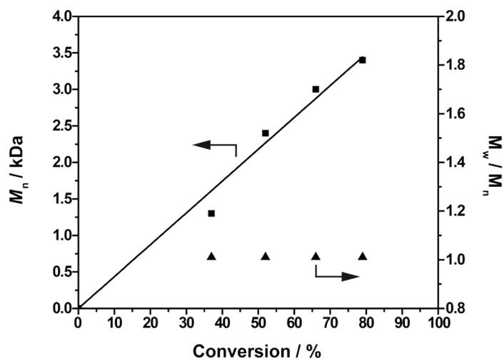
**Figure S35.** Evolution of  $M_n$  as a function of monomer conversion from the experiment in **Figure S34**.
