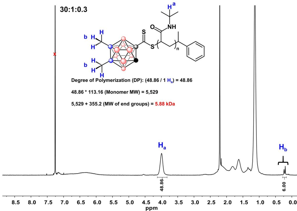
**Figure S16.**  $^1\text{H}$  NMR spectrum of 2-pNIPAAm in chloroform-*d* at 298 K and sample calculation of polymer molecular weight.
