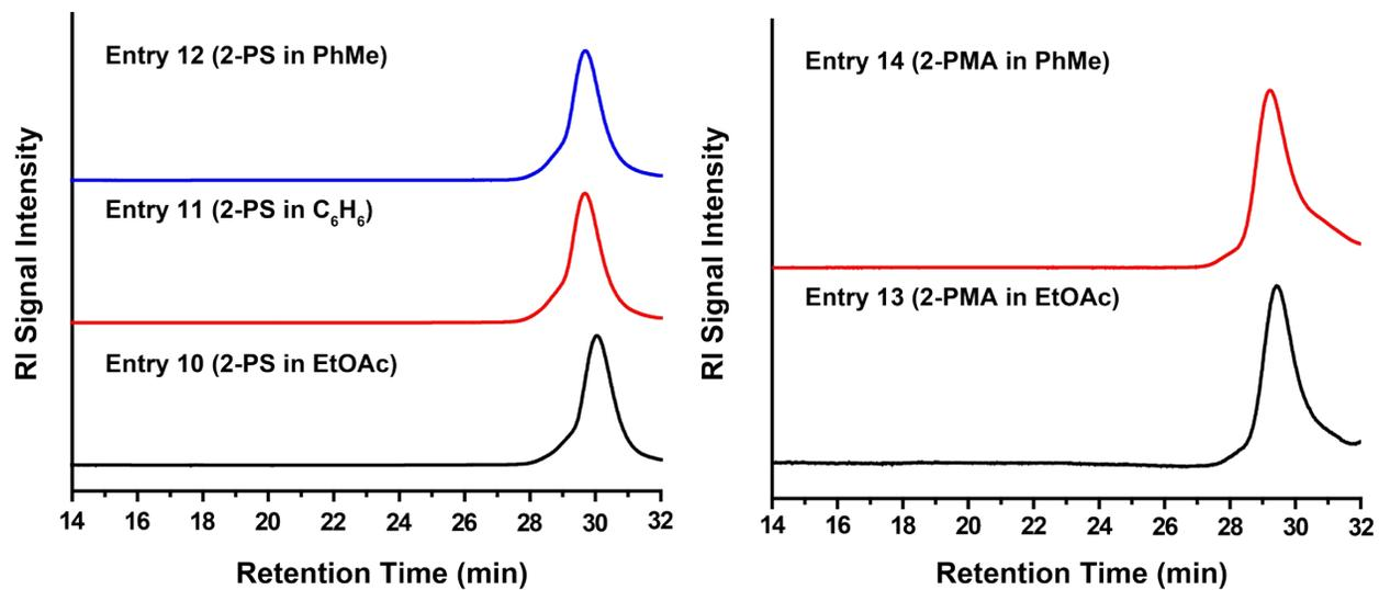
**Figure S26.** GPC traces of styrene and methyl acrylate in various solvents. GPC acquired using THF as the eluent.
