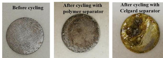
**Fig. S4** The optical photographs of the Li anodes harvested from the Li-S batteries before or after 200 cycles with different separators at 0.25C.
