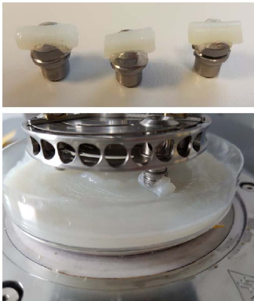
Figure S1. Digital image of MCR Tribometer set-up for tribological measurement, 3 cylindrical hydrogel samples were clamped to a T-PID/44 holder (top) and slid over a hydrogel sample prepared in a petri dish (below).
