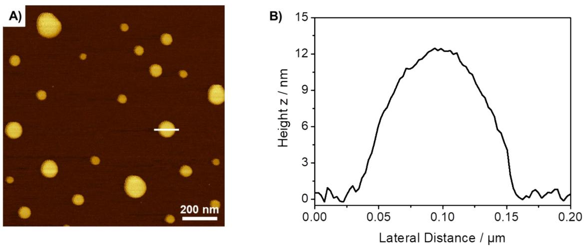
**Figure S8:** AFM height image (A), and cross-section (B) of Ba-PnBuA-TAP.
