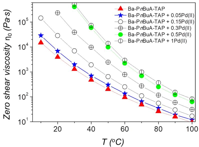
**Figure S6:** logarithmic plot of the zero shear viscosity  $\eta^0$  vs. temperature.
