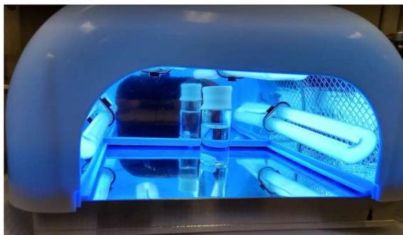
**Figure S1.** Photograph of the UV polymerization setup, consisting of 4 x 9 365 nm UV lamps and a custom made reflective cooling plate.
