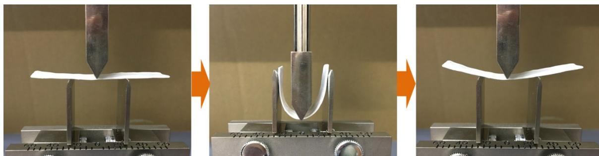
Figure S6. Photographs of a three-point bending test on VT21.
