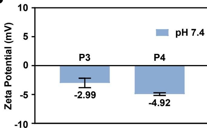
**Figure S3.** A) The size data (<sup>a</sup> These data show the systems are medium dispersion of particle size) and B) zeta potential values of P3/P4 in PBS buffer solution at pH 7.4. The average values and their standard deviations, from nine measurements, are shown.
