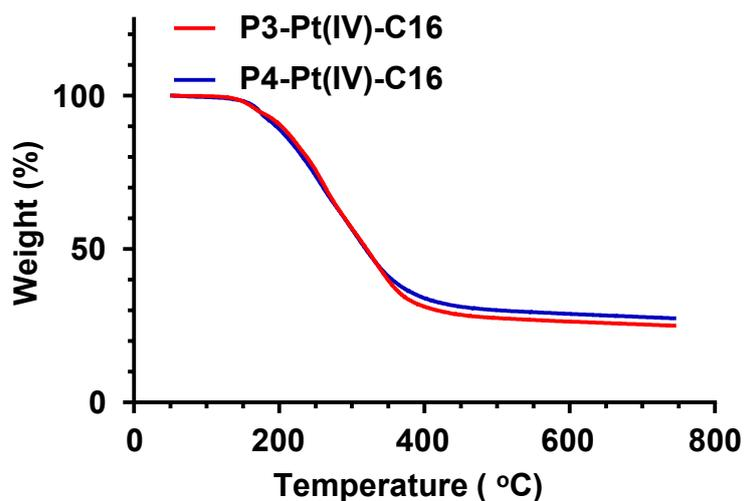
**Figure S6.** The thermostable curves of the lyophilized P3/P4-Pt(IV)-C16 nanoparticles analyzed by thermal gravimetric analyzer.
