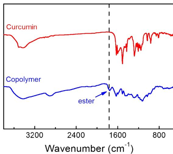
**Figure S1.** FT-IR spectra obtained for curcumin and poly(curcumin-*co*-oxalate) copolymers at 25 °C using KBr pellets.
