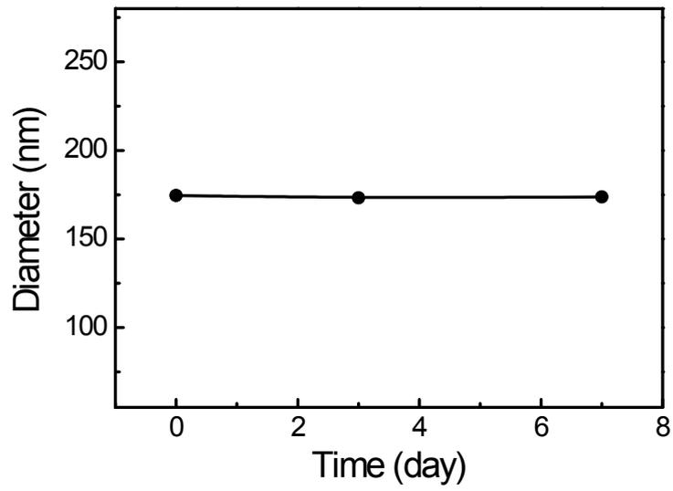
**Figure S4.** The time dependent size change of poly(curcumin-co-oxalate) nanoparticles measured in vitro by DLS in PBS buffer (pH 7.4) at 37 °C.
