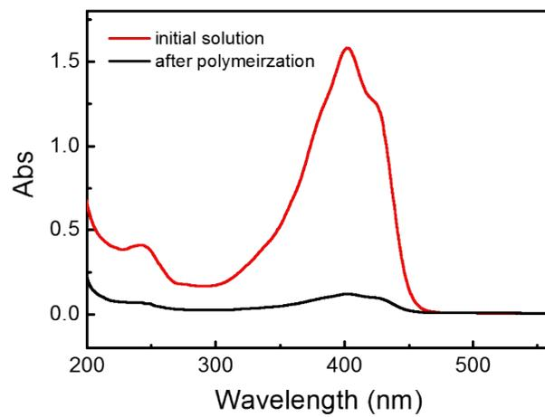
**Figure S2.** UV-vis spectra recorded for the mixture solution before and after polymerization, respectively.
