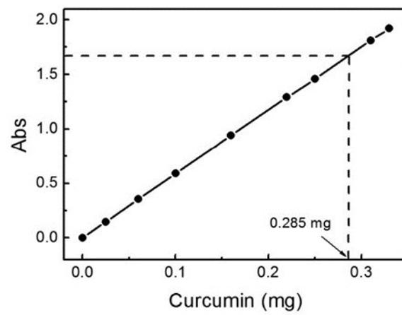
**Figure S3.** Concentration dependent absorption intensity of curcumin molecules in THF solution.
