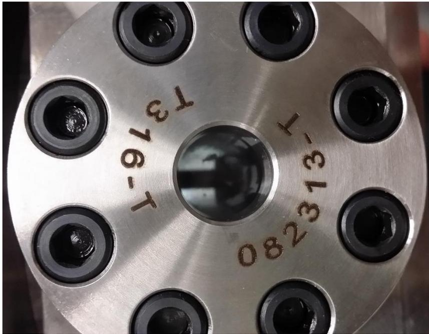
**S21.** Ethylene free radical polymerization in scCO<sub>2</sub> in the sapphire-windowed reactor.
