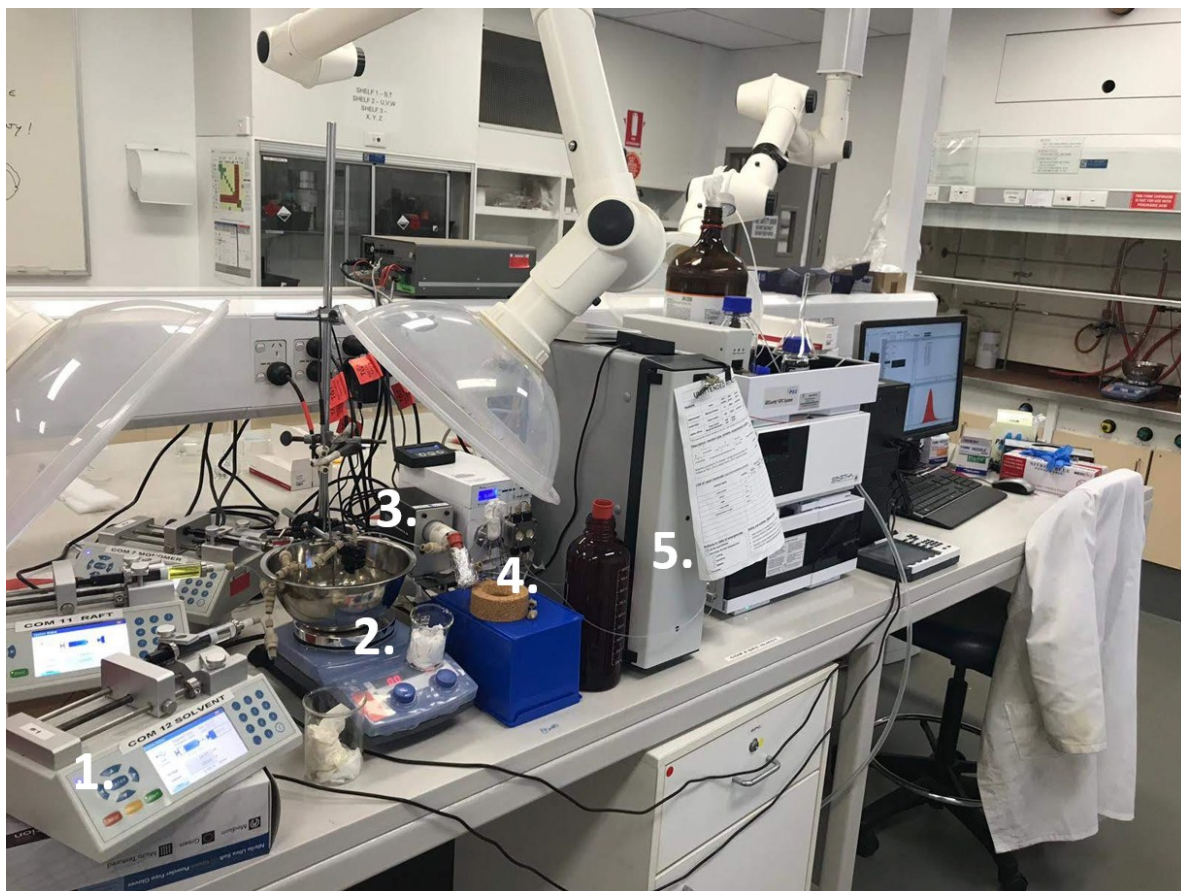
Figure 1: Overview of experimental setup to control molecular weight distribution through mixing. 1. Chemyx Fusion 100 syringe pumps. 2. Isothermal oil-bath containing continuous flow reactor. 3. Switch valve to direct product stream to online-GPC or collection to flask. 4. Collection vial. 5. Online-GPC setup used for the autonomous optimization to a predefined molecular weight.
