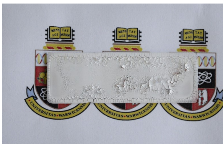
Figure S8. Film formation of the Sty/BA = 1.45:1 w:w latex made in presence of [NaCl] = 25.0 mM and dried at 40°C.
