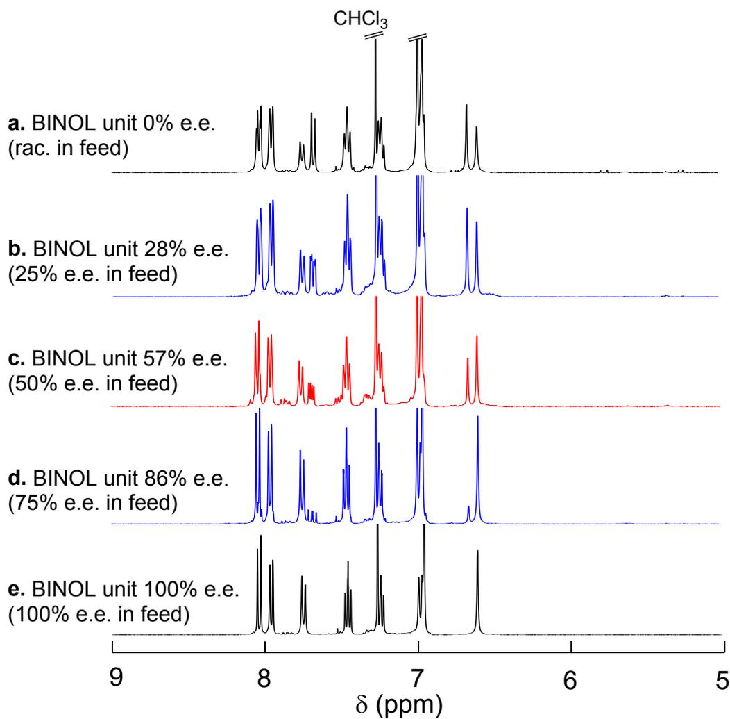
**Fig. S1.**  $^1\text{H}$  NMR spectra of BINOL-14DIB cyclic dimers (mixtures of R-R, R-S, S-S dimers) having different e.e.'s of BINOL units prepared at different e.e.'s of BINOL in feed and isolated by preparative SEC: BINOL unit e.e. 0% (a), 28% (b), 57% (c), 86% (d), and 100% (e) (pure R-R cyclic dimer). [400 MHz, r.t.,  $\text{CDCl}_3$ ]
