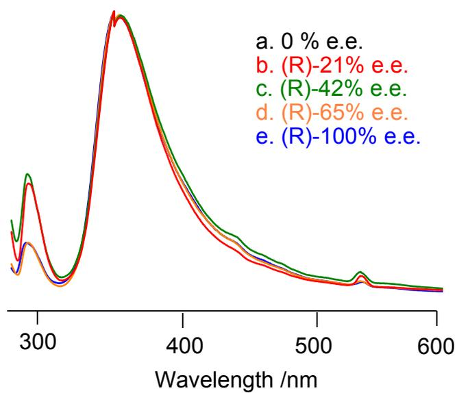
**Fig. S11.** Fluorescence spectra of poly(BINOL-*alt*-14DIB)s having different e.e.'s of BINOL units in a cast film: **a.** (R)-21% e.e.,  $M_n$  2920 (25% e.e. of (R)-BINOL in feed), **b.** (R)-42% e.e.,  $M_n$  2740 (50% e.e. of (R)-BINOL in feed); **c.** (R)-65% e.e.,  $M_n$  2870 (75% e.e. of (R)-BINOL in feed); **d.** (R)-100% e.e.,  $M_n$  3520; **e.** (R)- 0% e.e.,  $M_n$  2320.
