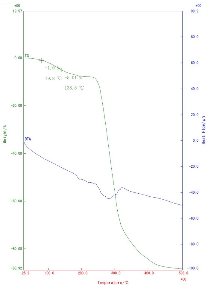
**Fig. S16.** DT-TGA profiles of poly(BINOL-*alt*-14DIB) ( $M_n$  2720) (A) and poly(BINOL-*alt*-13DIB) ( $M_n$  2460) (B) obtained at 100% e.e. of (*R*)-BINOL in feed [heating scan rate: 10 deg/min].
