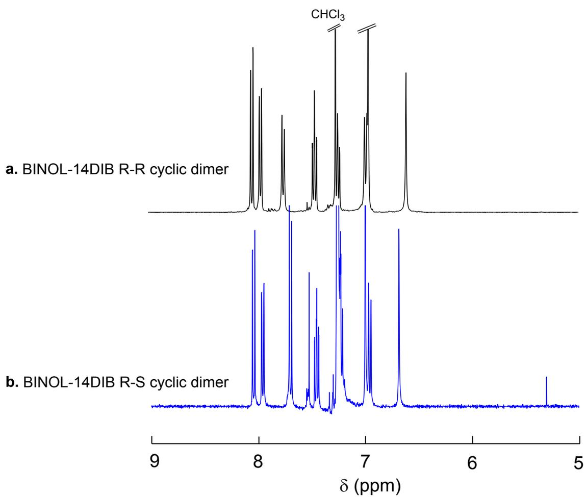
**Fig. S2.** <sup>1</sup>H NMR spectra of BINOL-14DIB cyclic dimers: pure R-R (a) and R-S cyclic dimers. [400 MHz, r.t., CDCl<sub>3</sub>]
