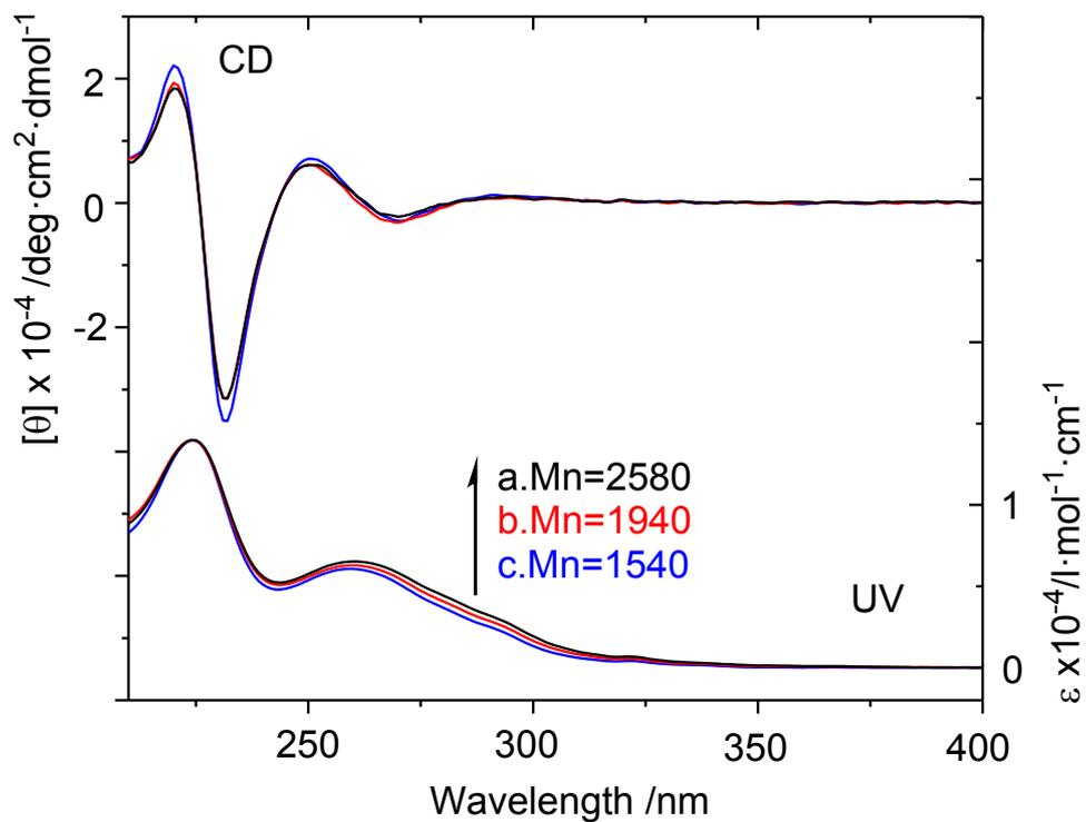
**Fig. S13.** UV and CD spectra of poly(BINOL-*alt*-14DIB)s of  $M_n$  2580 (a), 1940 (b) and 1540 (c) obtained at 50% e.e. of (*R*)-BINOL in feed in THF solution. The samples were separated from the product of reaction at  $[\text{BINOL}] = [\text{14DIB}] = -0.154 \text{ M}$  at room temperature for 24 h.
