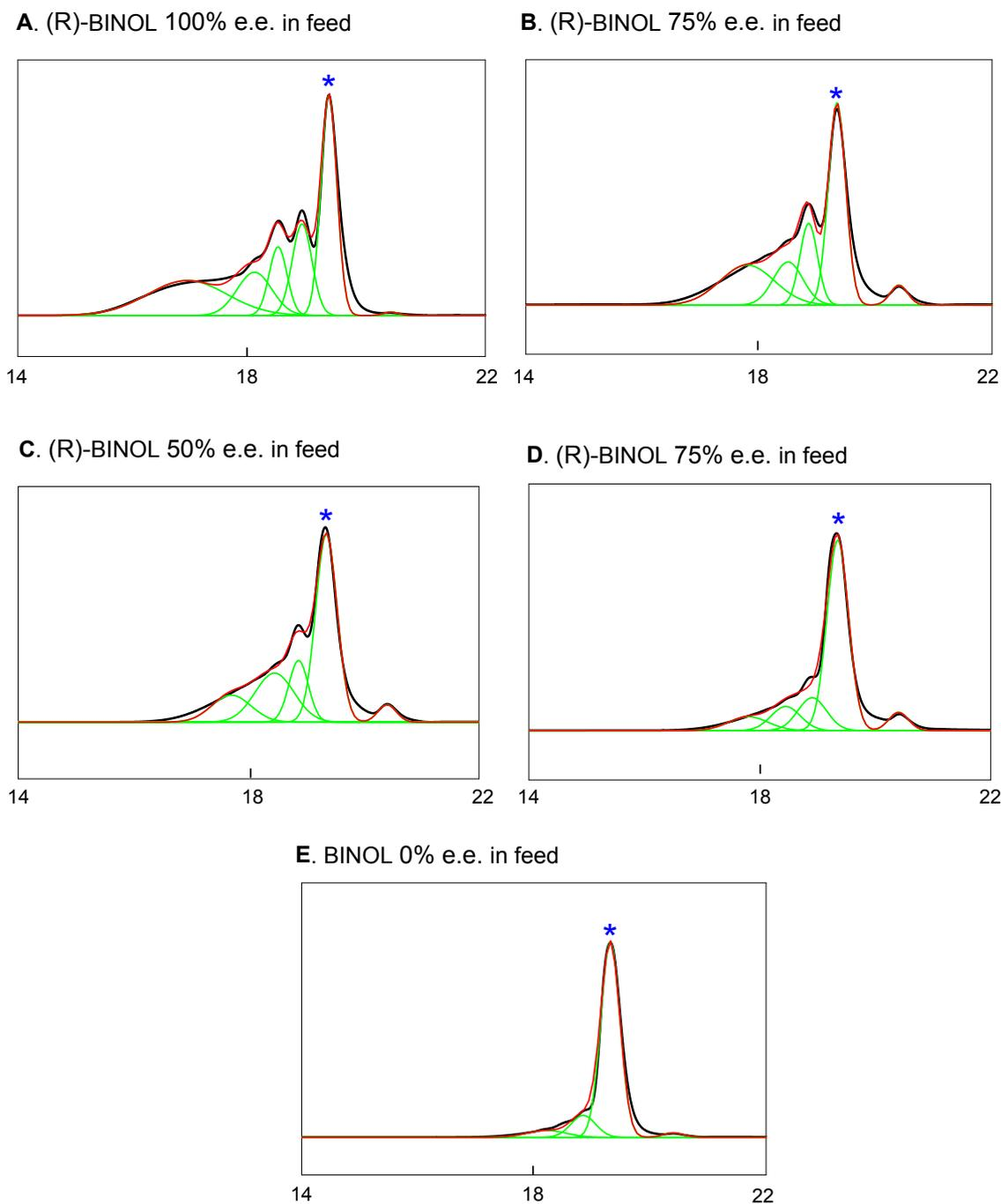
**Fig. S8.** Wave-form analysis of SEC curves of poly(BINOL-*alt*-14DIB) to determine the contents of cyclic dimer. Black curves are experimental SEC traces, green curves are deconvoluted Gaussian functions, and red curves are regenerated, entire SEC traces obtained by the addition of all deconvoluted functions. \* denotes cyclic dimer peaks.
