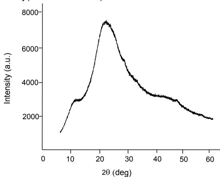
**Fig. S18.** WAXD profiles of poly(BINOL-*alt*-14DIB) ( $M_n$  2720) (A) and poly(BINOL-*alt*-13DIB) ( $M_n$  2460) (B). [RIGAKU Miniflex diffractometer, CuK $\alpha$ , 30 KV, 10 mA, scan speed 1.25 degree/min, step 0.01 degree]
