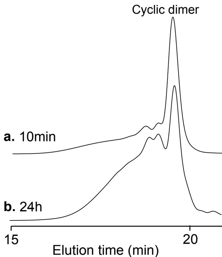
**Fig. S14.** SEC profiles of polymerization products obtained from 14DIB and (R)-BINOL at 50% e.e in 10 min (A) and 24 h (B) of reaction at  $[\text{BINOL}] = [\text{14DIB}] = 0.154 \text{ M}$  at room temperature. [detection by UV at 254 nm].
