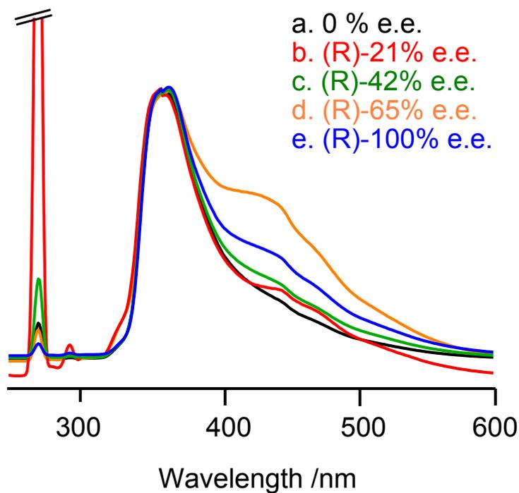
**Fig. S10.** Fluorescence spectra of poly(BINOL-*alt*-14DIB)s having different e.e.'s of BINOL units in a THF solution: **a.** (R)-21% e.e.,  $M_n$  2920 (25% e.e. of (R)-BINOL in feed), **b.** (R)-42% e.e.,  $M_n$  2740 (50% e.e. of (R)-BINOL in feed); **c.** (R)-65% e.e.,  $M_n$  2870 (75% e.e. of (R)-BINOL in feed); **d.** (R)-100% e.e.,  $M_n$  3520; **e.** (R)- 0% e.e.,  $M_n$  2320. [1-cm cell, conc.  $1.0 \times 10^{-3}$  M,  $\lambda_{ex}$  270 nm]
