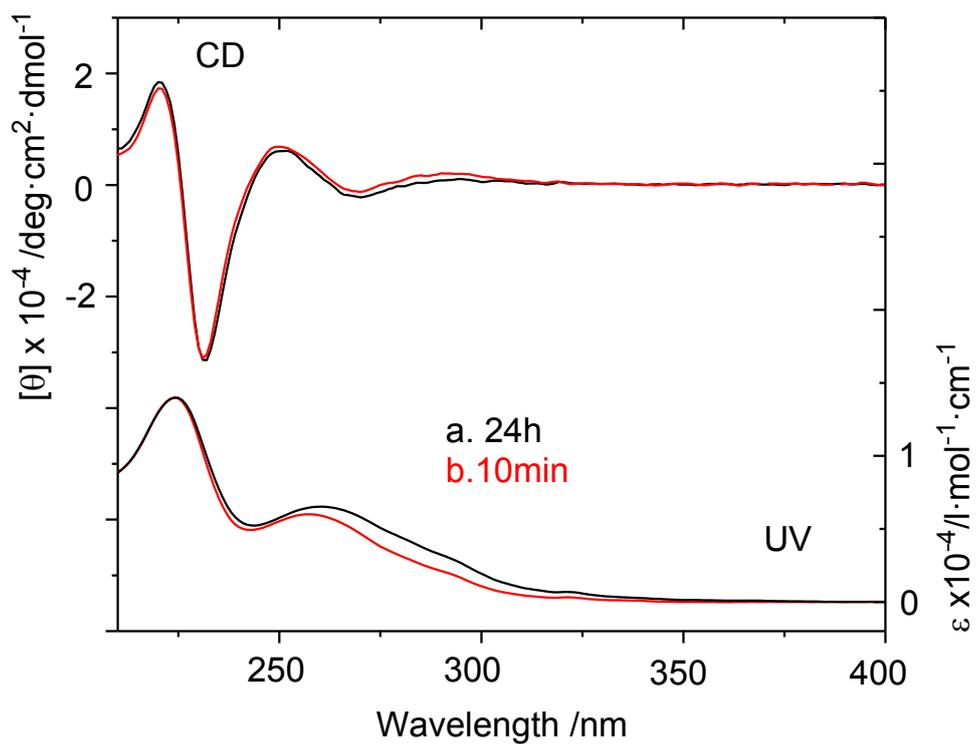
**Fig. S15.** UV and CD spectra of poly(BINOL-*alt*-14DIB)s obtained in 24 hn (a) and 10 min (b) of polymerization at 50% e.e. of (*R*)-BINOL in feed in THF solution.
