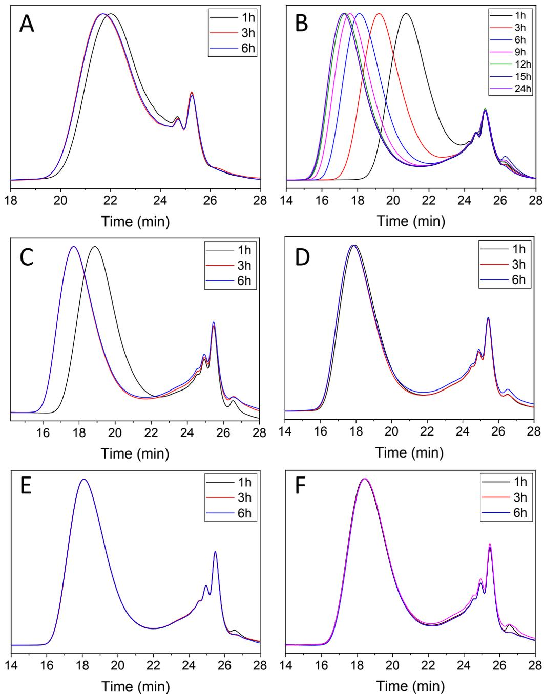
**Figure S7.** GPC curves of raw **Poly 1** prepared from a constant  $[M1]_0$  of 0.2 M and varied S ( $[DIBOD]_0/[M1]_0$ ) values of 0.91 (A), 1.0 (B), 1.1 (C), 1.2 (D), 1.5 (E), and 2.0 (F) at different reaction time. The polymerizations were all performed at room temperature in DMF. THF was used as eluent and polystyrene standards were used for calibration.
