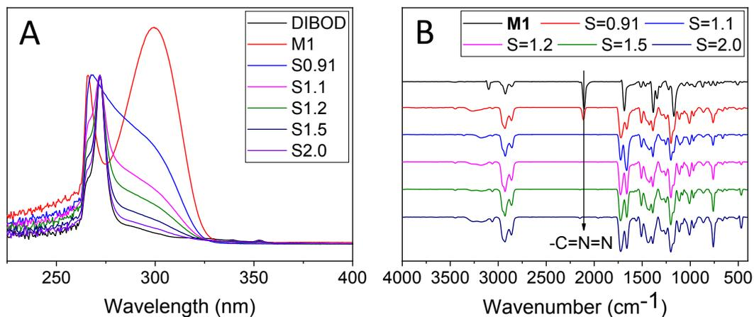
**Figure S8.** (A) UV-Vis spectra of DIBOD (black), **M1** (red), and raw **Poly 1** prepared from  $[M1]_0 = 0.2$  M and varied S ( $[DIBOD]_0/[M1]_0$ ) values of 0.91 (blue), 1.1 (magenta), 1.2 (olive), 1.5 (navy), and 2.0 (violet) in 3 h, where DMF was used as the measurement solvent. (B) FT-IR spectra of **M1** (black) and raw **Poly 1** prepared from  $[M1]_0 = 0.2$  M and varied S ( $[DIBOD]_0/[M1]_0$ ) values of 0.91 (red), 1.1 (blue), 1.2 (magenta), 1.5 (olive), and 2.0 (navy) in 3 h.
