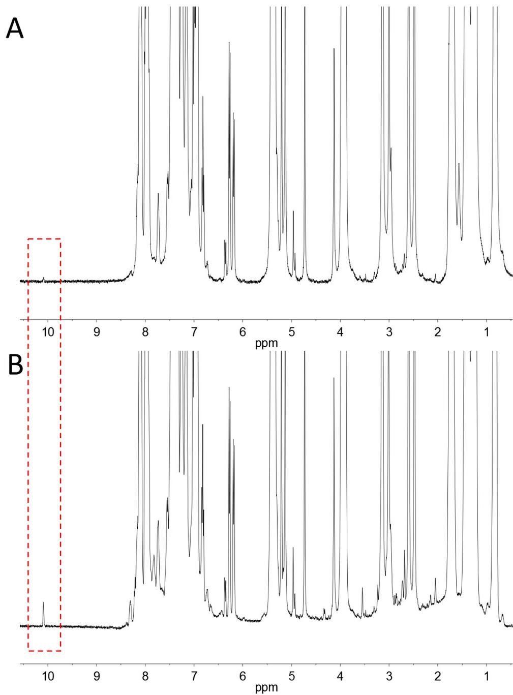
**Figure S28.**  $^1\text{H}$ -NMR spectra of the freshly precipitated **Poly 3-2** in  $\text{CDCl}_3$  (A) and the precipitated **Poly 3-2** storing in  $\text{CDCl}_3$  at room temperature after 4 days (B).
