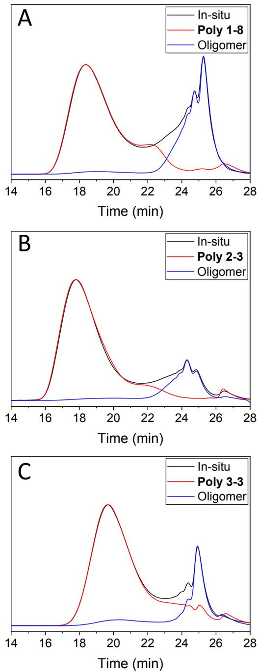
**Figure S9.** (A) GPC curves of raw **Poly 1-8** (black) and the corresponding high molecular weight **Poly 1-8** (red) and low molecular weight **Poly 1-8** oligomers (blue) separated from precipitation. (B) GPC curves of raw **Poly 2-3** (black) and the corresponding high molecular weight **Poly 2-3** (red) and low molecular weight **Poly 2-3** oligomers (blue) separated from precipitation. (C) GPC
