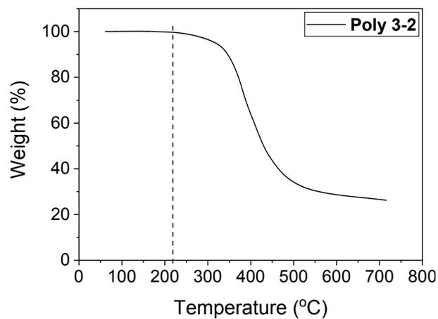
**Figure S27.** TGA curve of the freshly precipitated **Poly 3-2**, which was recorded with a heating rate of 10 °C/min under N<sub>2</sub>.
