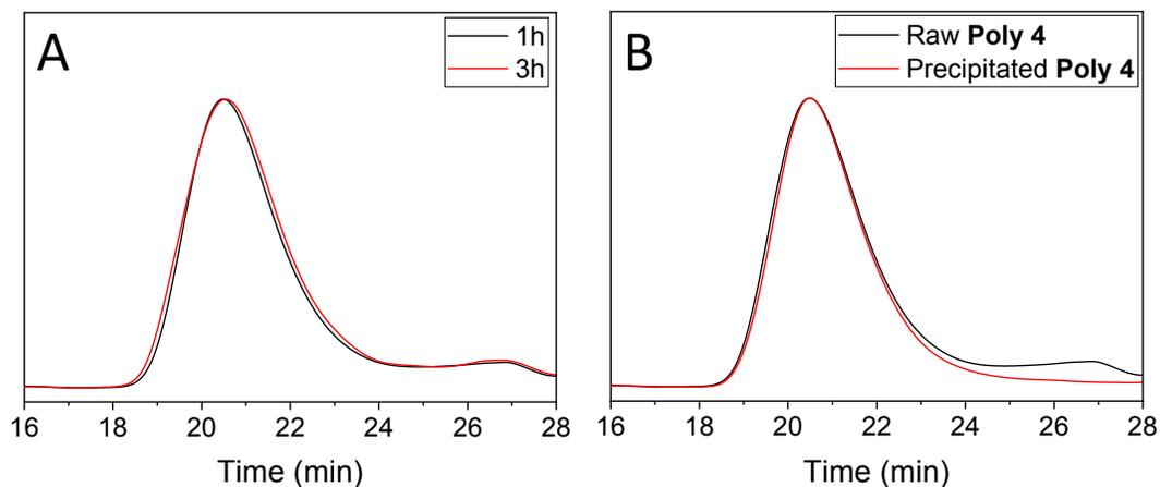
**Figure S20.** (A) GPC curves of the raw **Poly 4** prepared from  $[M4]_0 = 0.5$  M and S ( $[DIBOD]_0/[M4]_0 = 1.1$  in 1 h (black) and 3 h (red)). (B) GPC curves of the raw **Poly 4** (black curve) and precipitated **Poly 4** (red curve). DMF was used as the eluent and polystyrene standards were used for the calibration.
