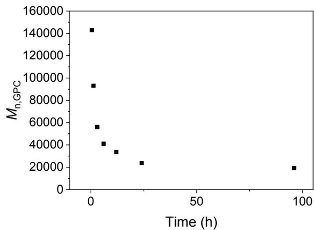
**Figure S24.** The relationship of  $M_{n, GPC}$  of degraded **Poly 3-2** and degradation time.
