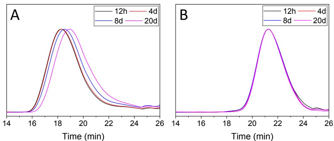
**Figure S25.** (A) GPC curves of the freshly precipitated **Poly 3-2** stored at room temperature for 12 h (black), 4 d (red), 8 d (blue), and 20 d (magenta). (B) GPC curves of the freshly precipitated **Poly 3-1** stored at room temperature for 12 h (black), 4 d (red), 8 d (blue), and 20 d (magenta). THF was used as the eluent and polystyrene standards were used for the calibration.
