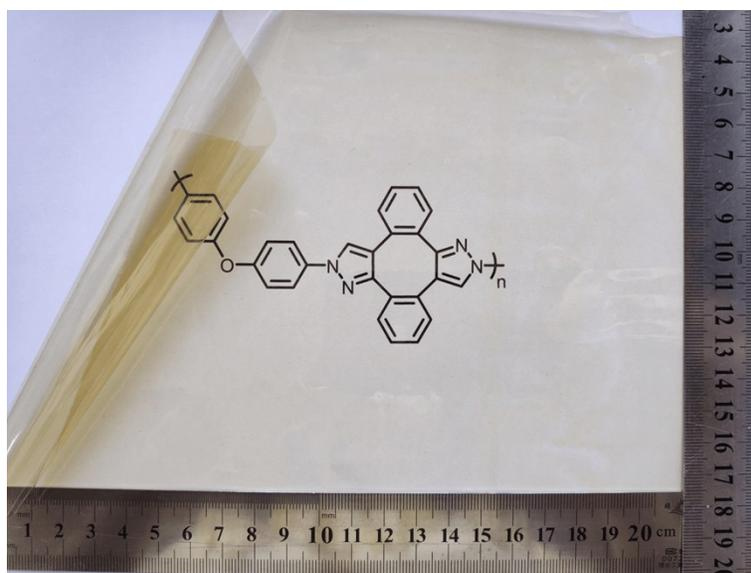
**Figure S23.** The photograph of thin film of precipitated **Poly 4**.
