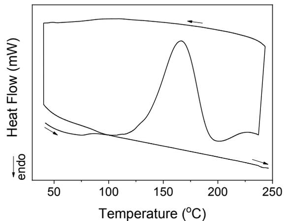
**Figure S26.** The DSC curve of the freshly precipitated **Poly 3-2**, which was recorded with a heating rate of 10 °C/min under N<sub>2</sub>.
