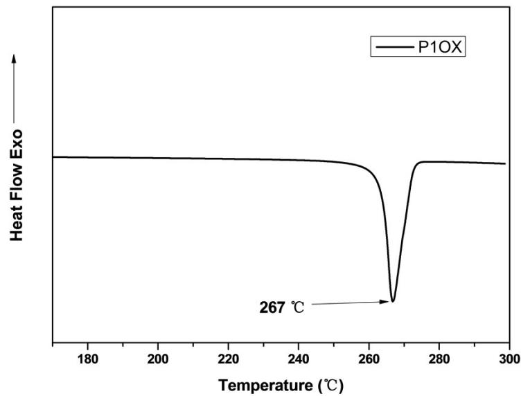
**Fig. S5** The melting point ( $T_m$ ) of P1OX measured by DSC.
