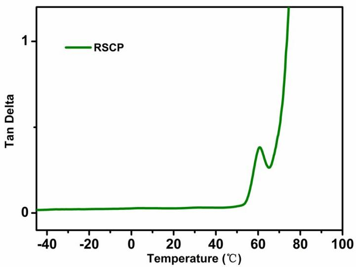
**Fig. S9** Overlay of tan  $\delta$  of RSCP determined by DMA.
