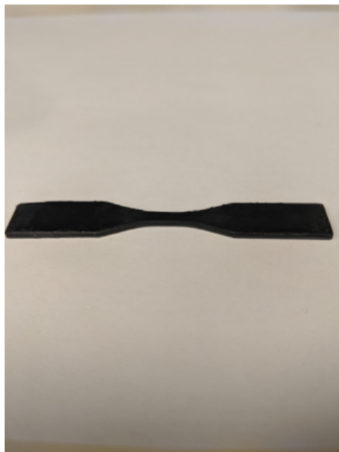
Fig. S6 Printed 10 mol% TAT ASTM D638 Type V dogbone unconditioned and after thermal conditioning at 200 °C for 2 hours. No significant changes in print structure were observed upon heating at these temperatures.
