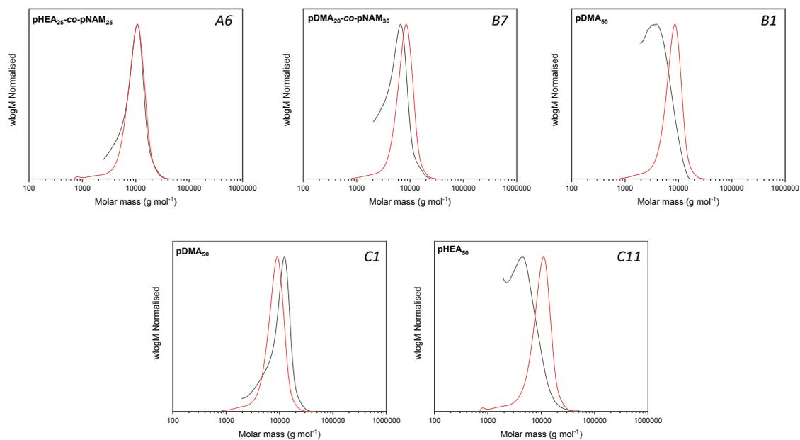
**Figure S6.** SEC chromatograms of pHEA<sub>25</sub>-co-pNAM<sub>25</sub> (Position A6), pDMA<sub>20</sub>-co-pNAM<sub>30</sub> (Position B7), pDMA<sub>50</sub> (Position B1), pDMA<sub>50</sub> (Position C1), pHEA<sub>50</sub> (Position C11) comparing the rapid-SEC (grey line) and conventional SEC (red line).
