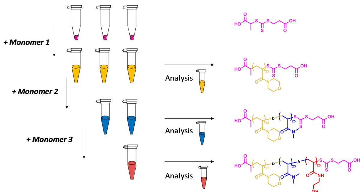
**Figure S4.** Schematic representation of the analysis method for preparing triblock copolymers via PCR-RAFT by removing a sample after each heating cycle.
