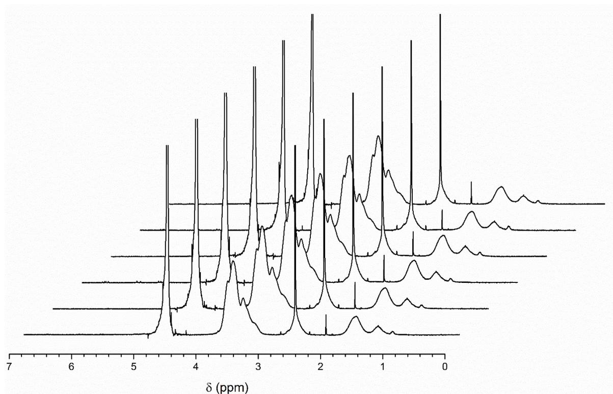
**Figure S3.**  $^1\text{H}$  NMR spectra in  $\text{D}_2\text{O}$  of the six  $\text{pNAM}_{50}$  prepared individually and heated in different wells of the 96 well thermocycler.
