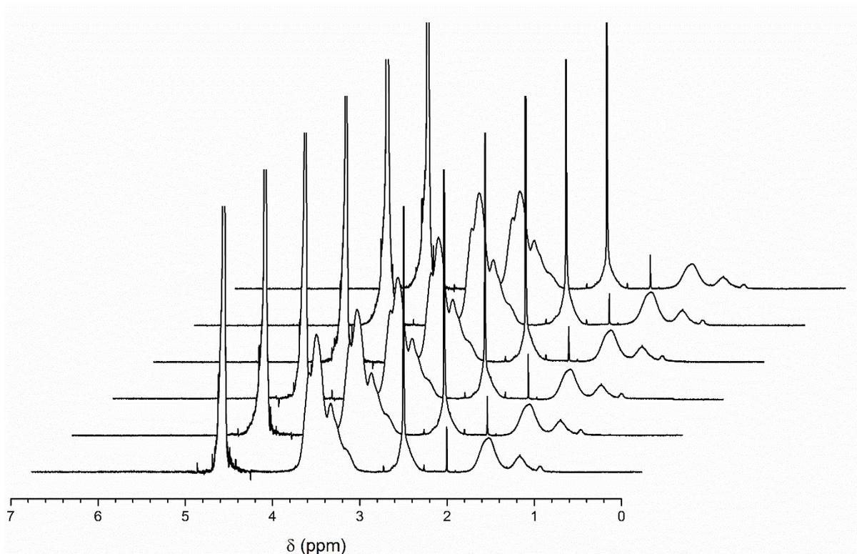
**Figure S2.**  $^1\text{H}$  NMR spectra in  $\text{D}_2\text{O}$  of the six  $\text{pNAM}_{50}$  prepared from same mother solution, aliquoted and heated in different wells of the 96 well thermocycler.
