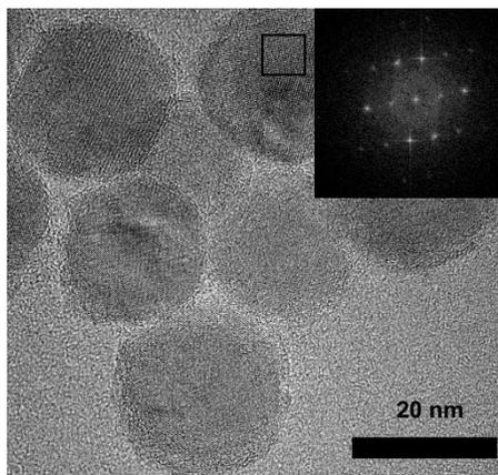
High resolution transmission electron micrograph, scale bar is 20 nm. Inset showing fast Fourier transform of the area outlined in the box showing lattice fringes indicative of crystallinity.
