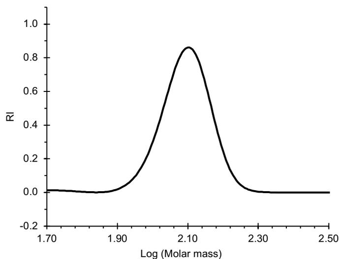
Gel permeation chromatogram (GPC) of cleaved BAAM polymer from MNPs.  $M_n=71.2$  kDa  $M_w=115$  kDa and polydispersity index of 1.62. The polymer corresponds to BAAM-MNP-86.
