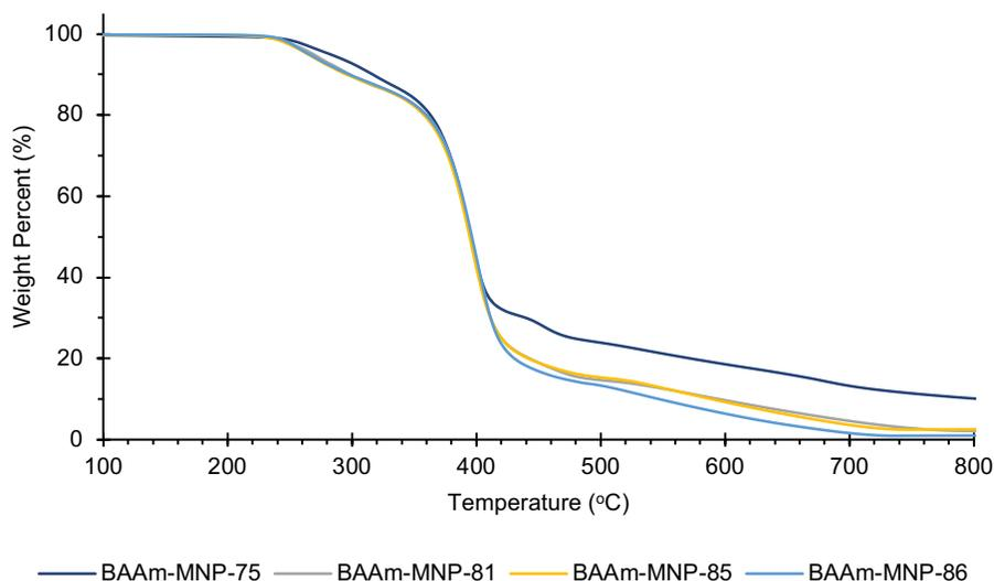
Thermogravimetric Analysis (TGA) was conducted on TA Instruments Q500 TGA. Samples were equilibrated at 100 °C for 30 minutes under nitrogen, followed by a temperature ramp of 10 °C/min to 800 °C.
