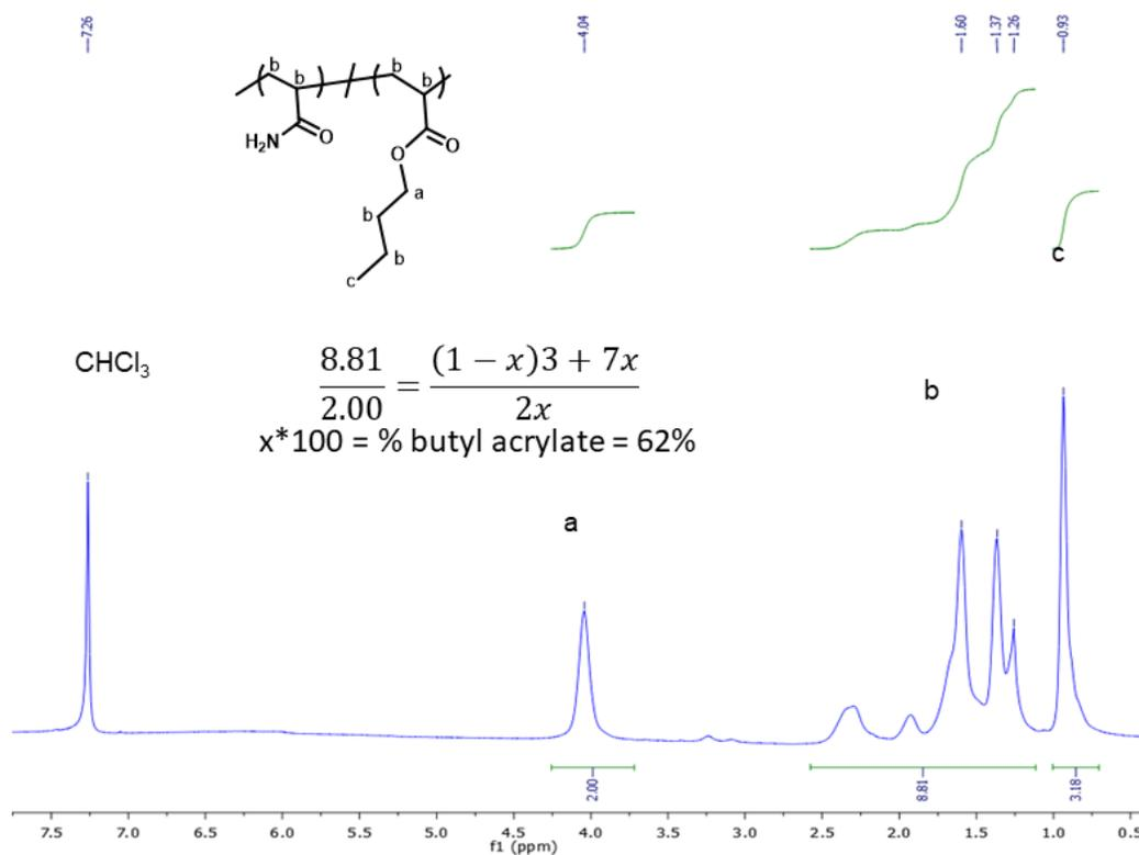
NMR analysis of BAAM-MNP-86 after cleaving from MNP using hydrofluoric acid. The calculation for percent incorporation of butyl acrylate is shown above. The percent incorporation of butyl acrylate is 62% and for acrylamide it's 38% given a feed ratio of 60% and 30% of butyl acrylate and acrylamide, respectively.
