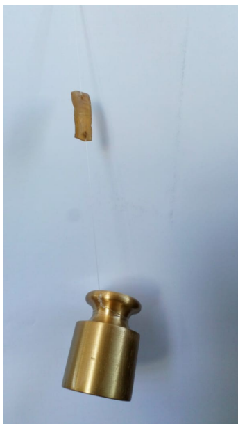
Fig. 6S. Welded epoxy vitrimer based on HA after 1 h at 120 °C, supporting a 300 g weight.
