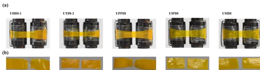
**Fig. S7** The UHDI-1, UTDI-2, UPPDI, UIPDI and UMDI film (a) during stretching and (b) after fracture at a strain rate of  $5 \text{ s}^{-1}$ .
