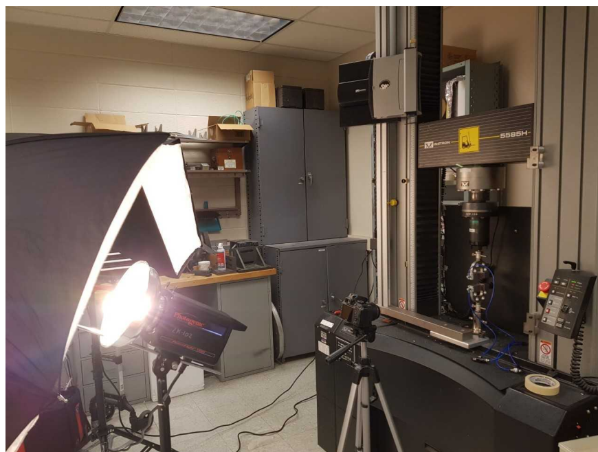
Figure S13. Camera setup (with lighting setup of S9) for taking images of SP-PDMS samples (with black background). Nikon camera was used.
