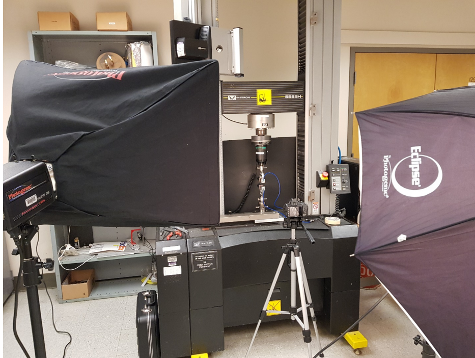
Figure S14. Camera and lighting setup for taking images of SP-PDMS samples (with black background).
