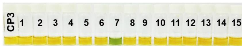
**Figure S2.** Color of CP3 solution upon treatment with several interfering cations: 1 ( $Mg^{2+}$ ), 2 ( $As^{3+}$ ), 3 ( $Zn^{2+}$ ), 4 ( $Mn^{2+}$ ), 5 ( $Na^+$ ), 6 ( $Hg^{2+}$ ), 7 ( $Cu^{2+}$ ), 8 ( $K^+$ ), 9 ( $Cd^{2+}$ ), 10 ( $Ni^{2+}$ ), 11 ( $Ca^{2+}$ ), 12 ( $Co^{2+}$ ), 13 ( $Cr^{3+}$ ), 14 ( $Fe^{2+}$ ), 15 ( $Fe^{3+}$ ).
