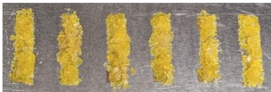
Figure S17. Image of ground PO 23% - grad network in the dogbone mold. Unintentionally, no image was taken directly after reprocessing.
