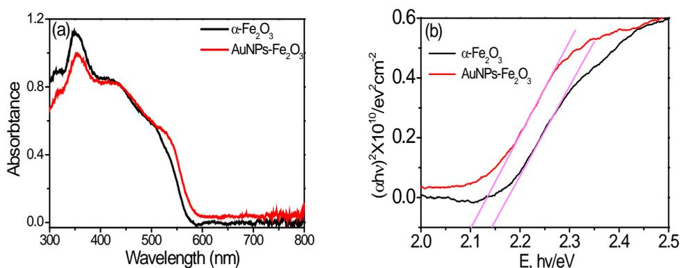
Fig. S8 (a) UV-Vis spectra of  $\alpha$ -Fe<sub>2</sub>O<sub>3</sub> and AuNPs-Fe<sub>2</sub>O<sub>3</sub> and (b) Band gap values of  $\alpha$ -Fe<sub>2</sub>O<sub>3</sub> and AuNPs-Fe<sub>2</sub>O<sub>3</sub>
