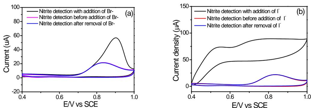
Fig. S9 Selectivity of the sensor for nitrite over other ions in PBS solutions (pH = 7.0) containing 50  $\mu$ M nitrite in the presence of: (a) 2.5 mM Br<sup>-</sup> and (b) 0.5 mM of I<sup>-</sup>
