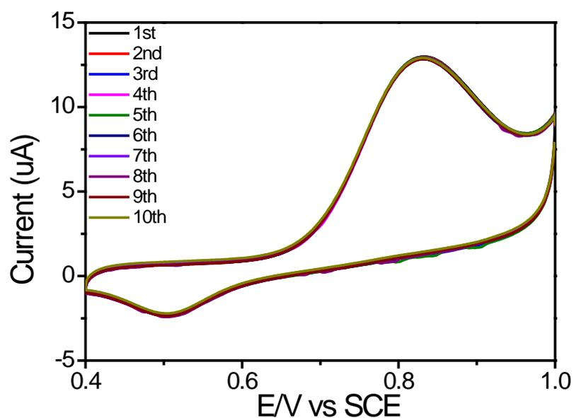
Fig. S10 Reproducibility of nitrite sensor with AuNPs- $Fe_2O_3$  photoelectrode
