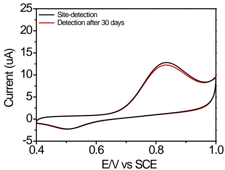
Fig. S12 CV curves of storage stability by the fabricated sensor with AuNPs-Fe<sub>2</sub>O<sub>3</sub> photoelectrode. Condition: 50  $\mu\text{M}$  NO<sub>2</sub><sup>-</sup> in PBS solution (pH = 7), scan rate potential of 50  $\text{mv}\cdot\text{s}^{-1}$ , and using the same electrode after 30 days of storage at ambient temperature for nitrite detection.
