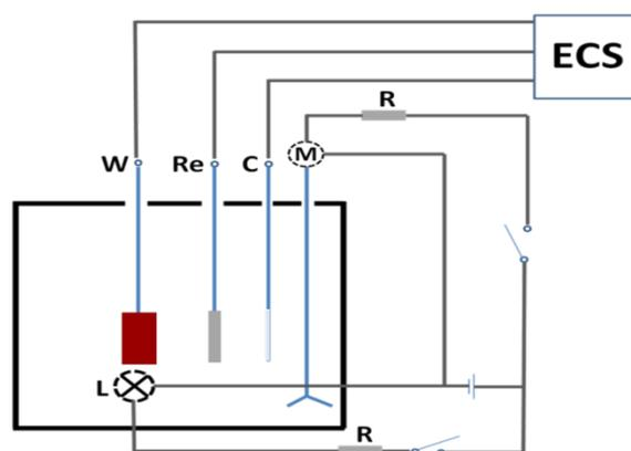
Fig. S4 Schematic illustration of device for nitrite detection
