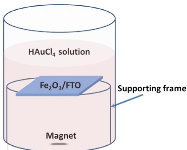
Fig. S1 Simple device for synthesis of AuNPs- $\text{Fe}_2\text{O}_3$  thin-film nanocomposite.
