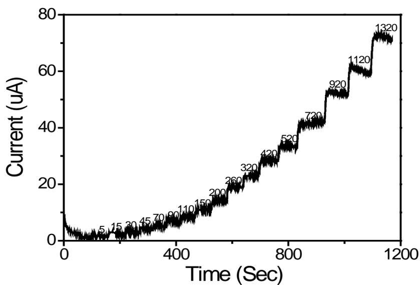
Fig. S5 Amperometric response of AuNPs-Fe<sub>2</sub>O<sub>3</sub> electrode under the absence of light at an operating potential of 0.83 V (vs. SCE) with the addition of NO<sub>2</sub><sup>-</sup> to 0.1 M PBS buffer solution (pH = 7.0).
