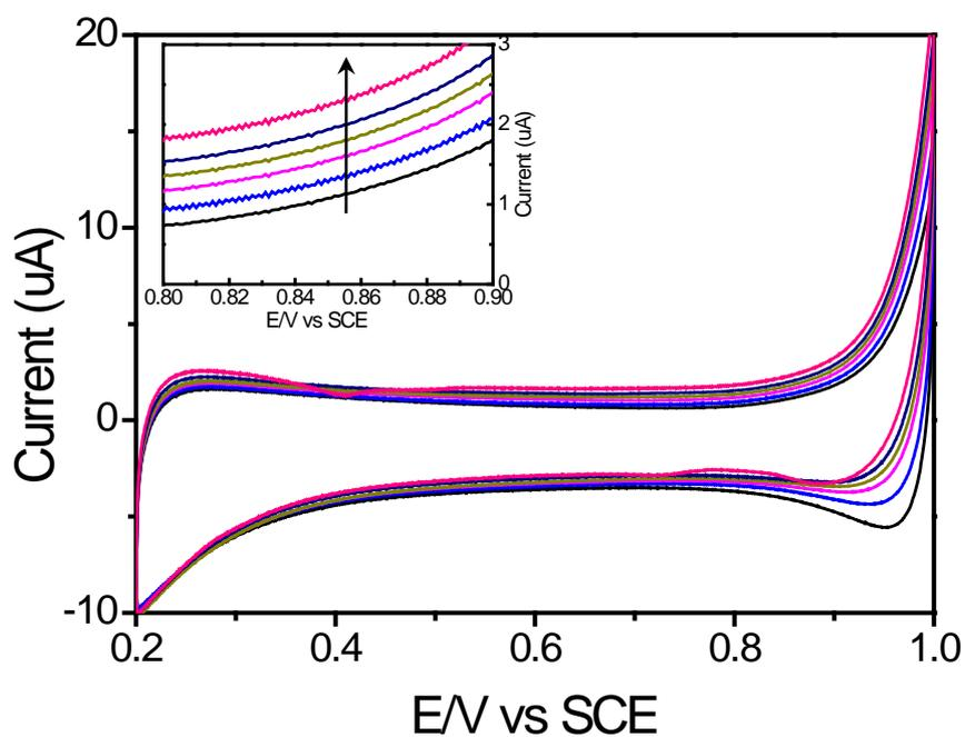
Fig. S6 CV curves with  $\alpha$ -Fe<sub>2</sub>O<sub>3</sub> electrode at various nitrite concentrations from 50  $\mu$ M to 1000  $\mu$ M under illumination.
