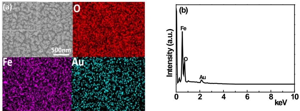
Fig. S3 (a) elemental mappings of O, Fe, and Au (Topleft: selected area in box for mapping, topright: oxygen distribution, bottom left: iron distribution and bottom right: gold distribution); (b) EDX curves for the AuNPs-Fe<sub>2</sub>O<sub>3</sub>.
