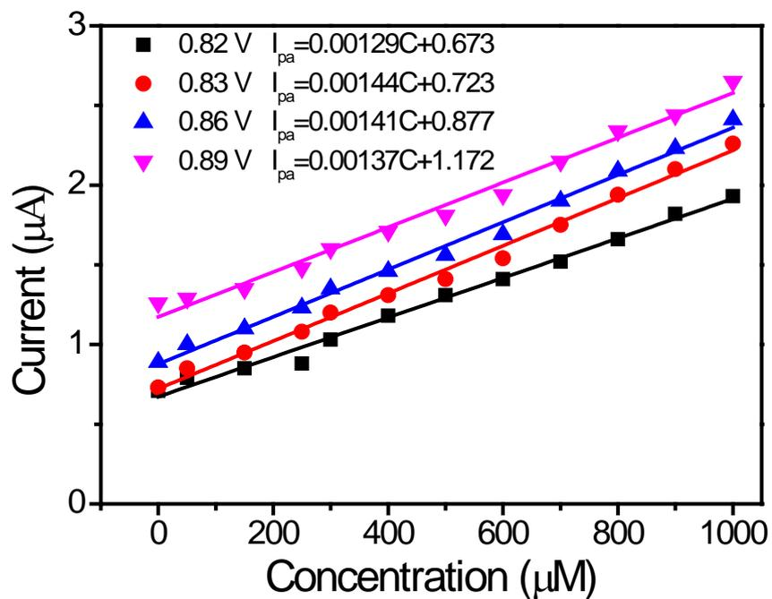
Fig. S7 Linear fitting by the plot of current vs. nitrite concentration under different potential (data from Fig.
