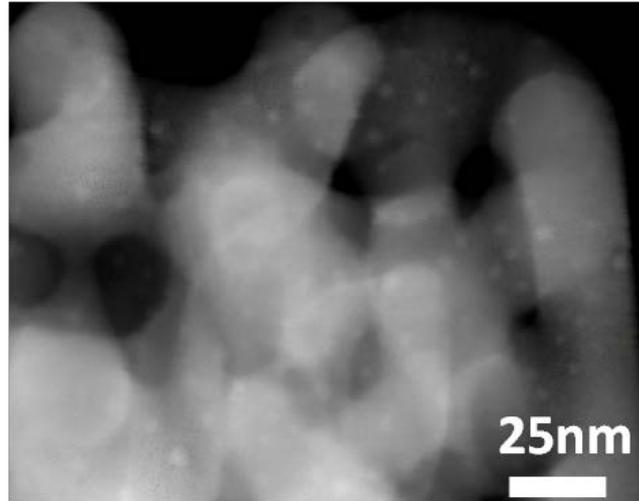
Fig. S2 TEM image of AuNPs-Fe<sub>2</sub>O<sub>3</sub> NRAs.
