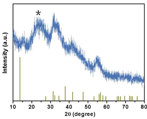
Figure S11. XRD pattern of the 1.93 wt% Ru-WSe<sub>2</sub> nanosheets after chronopotentiometry test (\* represents the peak of XC-72).
