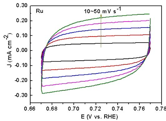
Figure S9. Electrochemical double layer capacitance curves on Ru nanorods with different scan rates from 50  $\text{mV s}^{-1}$  to 10  $\text{mV s}^{-1}$  in 1.0 M KOH.
