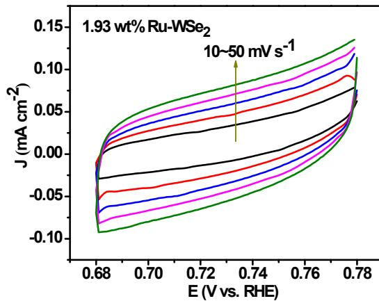
Figure S8. Electrochemical double layer capacitance curves on 1.93 wt% Ru-WSe<sub>2</sub> with different scan rates from 50  $\text{mV s}^{-1}$  to 10  $\text{mV s}^{-1}$  in 1.0 M KOH.
