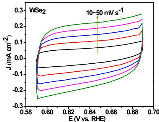
Figure S10. Electrochemical double layer capacitance curves on WSe<sub>2</sub> with different scan rates from 50  $\text{mV s}^{-1}$  to 10  $\text{mV s}^{-1}$  in 1.0 M KOH.
