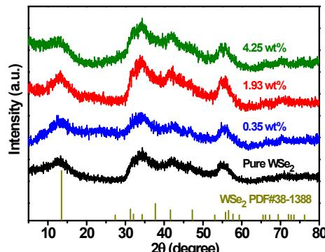
Figure S1. The XRD patterns of Ru-WSe<sub>2</sub> nanocomposites with different contents of Ru and pure WSe<sub>2</sub>.
