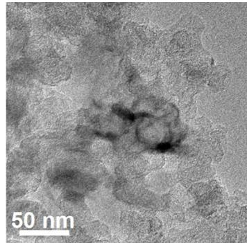
Figure S12. TEM image of the 1.93 wt% Ru-WSe<sub>2</sub> nanosheets after chronopotentiometry test.
