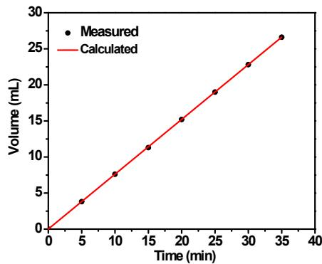
Figure S13. The amount of hydrogen theoretically calculated and experimentally measured versus time for 1.93 wt% Ru-WSe<sub>2</sub> in 1.0 M KOH.
