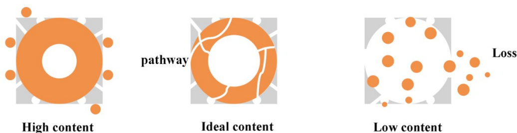
Figure S14. The mechanism diagram of Se content impact on electrochemical performance.
