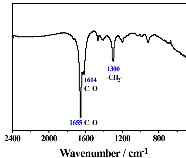
**Figure S1** Infrared spectrum of C4Q
