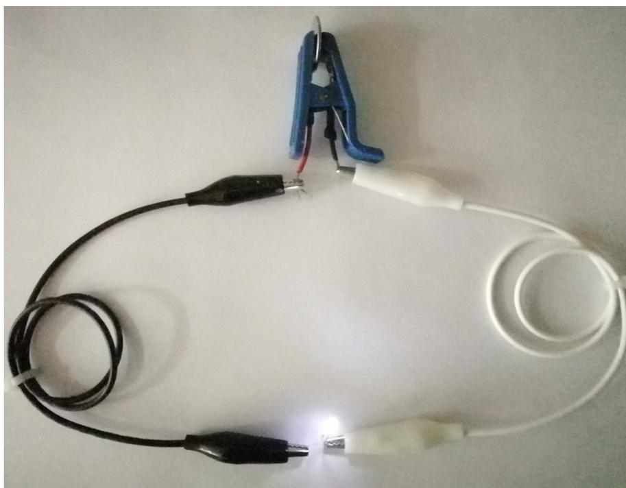
Fig. S6 Photo of white LED bulb lighted up by  $\text{Na}_3\text{V}_2(\text{PO}_4)_3$ //SNCT-2 full cell SIB.
