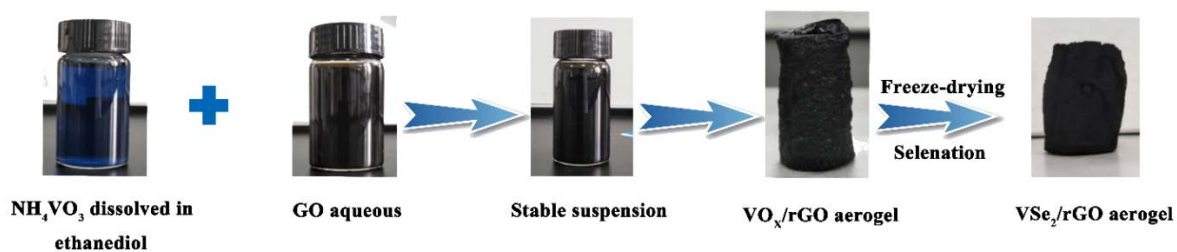
Fig. S1 Schematic illustration of the route for synthesis of 3D VSe 2 /rGO aerogel.
