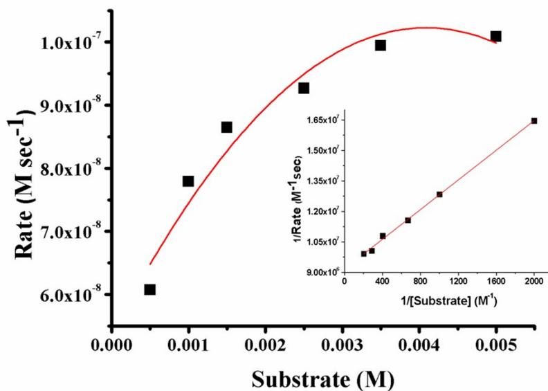
**Fig. S10** Plot of the initial rates vs substrate concentration for the oxidation of 3,5-DTBC catalyzed by **1**. The inset shows Lineweaver–Burk plot.
