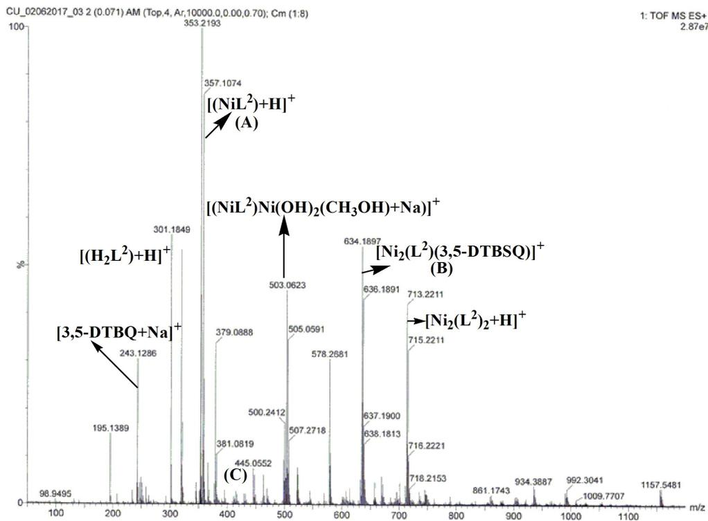
Fig. S13 ESI-MS spectrum of **3** with 3,5-DTBC in methanol.
