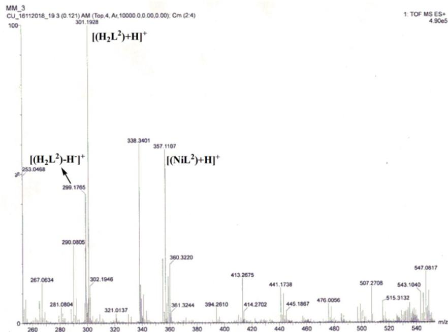
**Fig. S7** ESI-MS spectrum of the 1:1:4 molar mixture of **1**, purified nickel perchlorate complex of the unreduced ligand and NH<sub>4</sub>SCN taken after one week in methanol.
