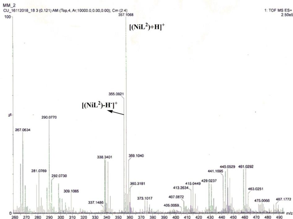
**Fig. S6** ESI-MS spectrum of the 1:1 molar mixture of **1** and purified nickel perchlorate complex of the unreduced ligand taken after one week in methanol.
