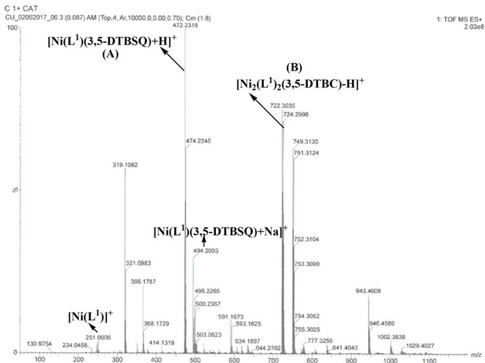
Fig. S12 ESI-MS spectrum of **1** with 3,5-DTBC in methanol.
