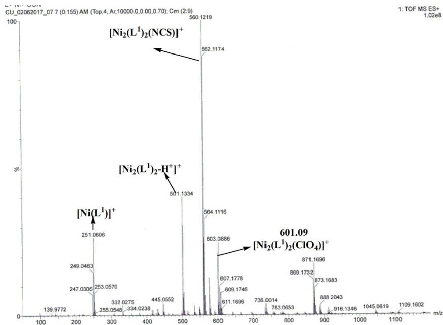
**Fig. S5** ESI-MS spectrum of reaction mixture in methanol taken immediately after mixing *in situ* generated **1** and  $\text{NH}_4\text{SCN}$  in 1:2 ratios.
