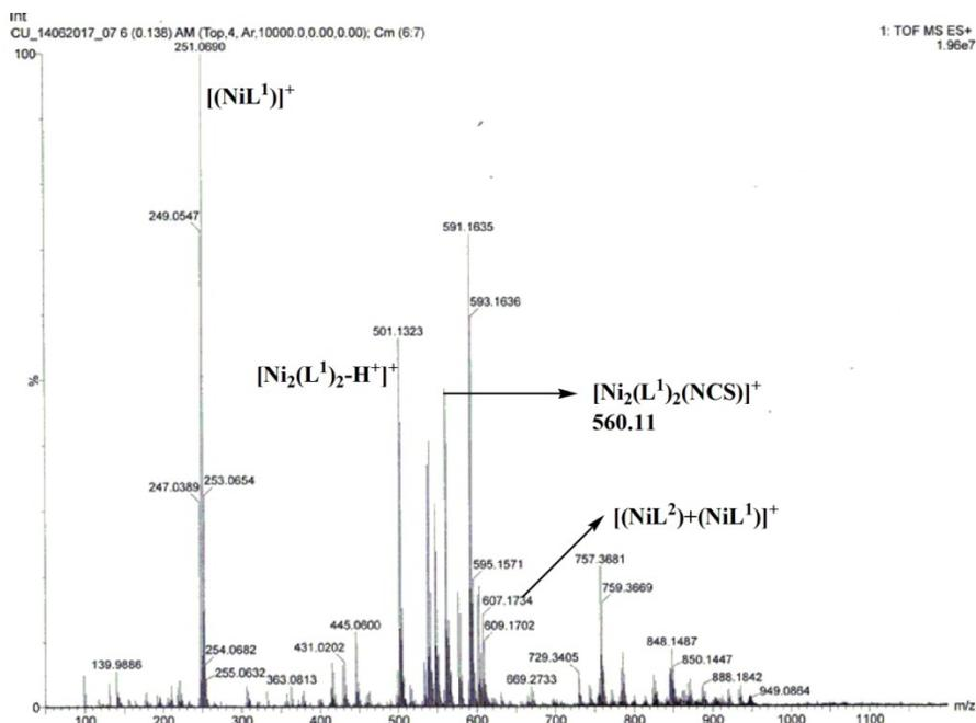
**Fig. S8** ESI-MS spectrum of the 1:2 molar mixture of **1** and  $\text{NH}_4\text{SCN}$  taken after one week in methanol.
