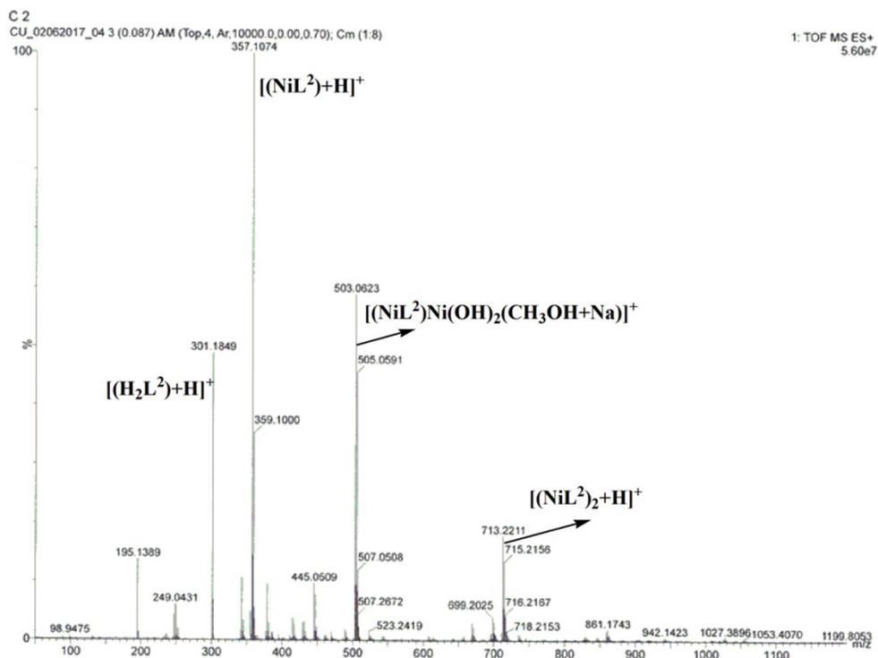
Fig. S2 ESI-MS spectrum of **2** in methanol.
