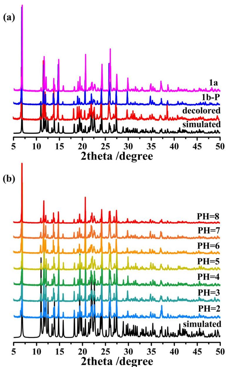
**Fig. S4** (a) Simulated and experimental PXRD patterns of **1**. (b) PXRD patterns of samples soaking in pH = 2–8 water solution for 24 h. Labels: **1a**: before irradiation; **1b-P**: after photo irradiation; decolored: heating in 50 °C for 20 min.
