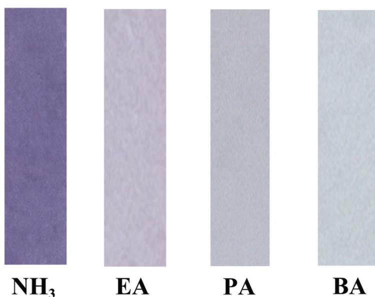
**Fig. S12** Portable test strips for visual and differentiable detection of amines. Labels: EA, PA, BA, NH<sub>3</sub>, **1a** exposed to ethamine, n-propylamine, n-butylamine, NH<sub>3</sub>.
