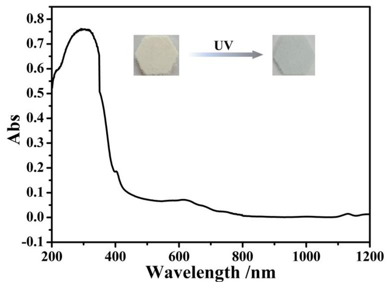
**Fig. S9** UV-Vis diffuse reflectance spectra of the crystal samples upon UV light irradiation with intensity of 0.001 mW/cm<sup>2</sup>. The colors change was shown in the inset before and after photo-irradiation.
