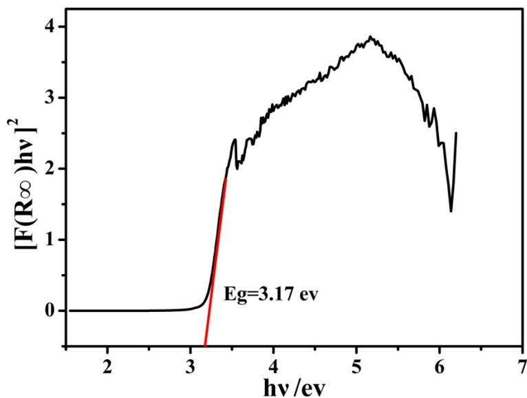
**Fig. S6** Optical band gap energy of compound **1**.
