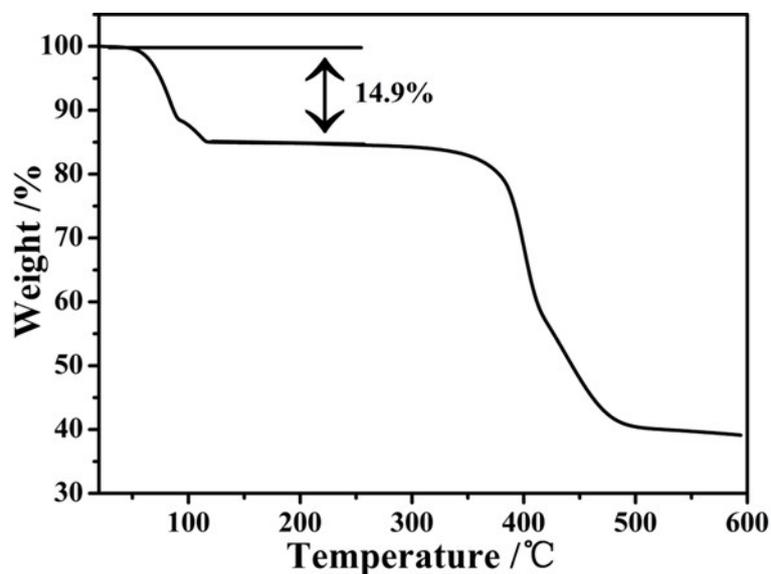
**Fig. S13** TGA curve of **1** was investigated using powder samples under  $N_2$ . The weight loss is 14.9 % (calcd 15.1 %) up to 116 °C corresponding to the loss of three free  $H_2O$  and one coordinated  $H_2O$ .
