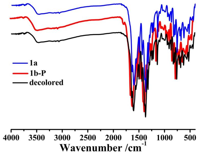
**Fig. S5** FT-IR spectra of **1**. Labels: **1a**: before irradiation; **1b-P**: after photo irradiation; **decolored**: heating in 50 °C for 20 min.
