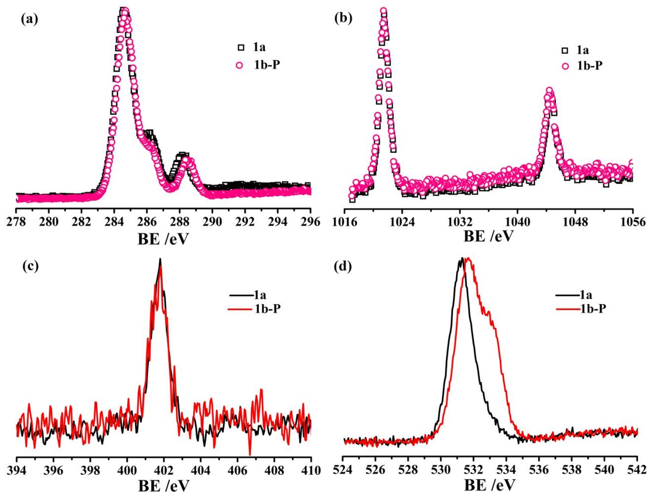
Fig. S8 XPS (Al- $K\alpha$ ) core-level spectra of compound **1** for C 1s (a), Zn 1s (b), N 1s (c) and O 1s (d) before and after photo irradiation in a vacuum. Labels: **1a**, before irradiation; **1b-P**, after photo irradiation; BE: Binding Energy.
