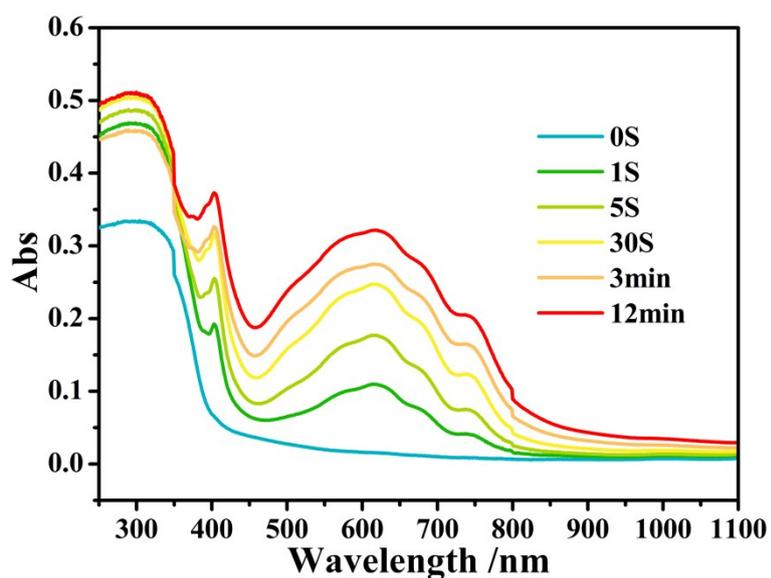
**Fig. S14** Time-dependent UV-Vis diffuse reflectance spectra of **1** upon 300 W ultraviolet light irradiation at room temperature in air.
