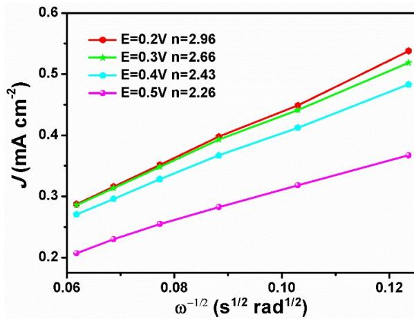
**Figure S21.** Corresponding K–L plots at different potentials of **SOF-21/CB**.
