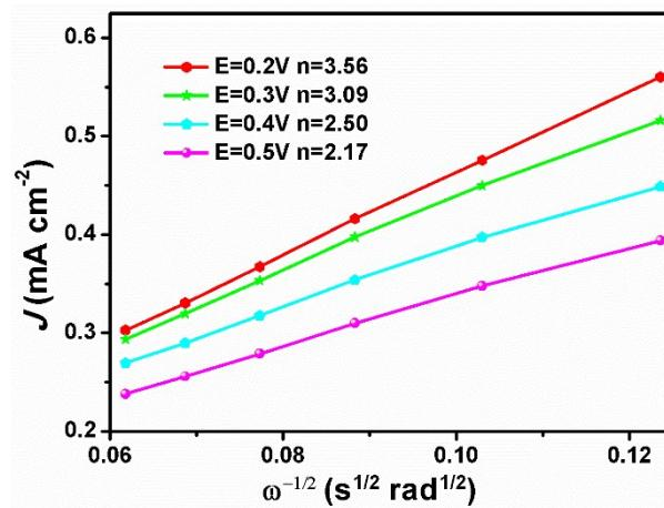
**Figure S20.** Corresponding K–L plots at different potentials of **SOF-20/CB**.
