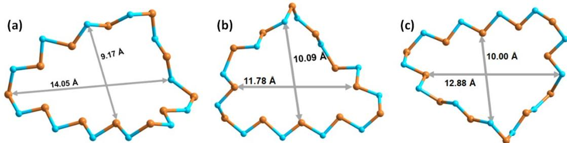
**Figure S7.** Three kinds of 24-MR windows observed in **SOF-20**: (a) window A; (b) window B; (c) window C.
