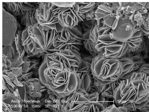
Fig. S2 SEM image of the  $\text{VS}_2 \cdot \text{NH}_3$  precursor.
