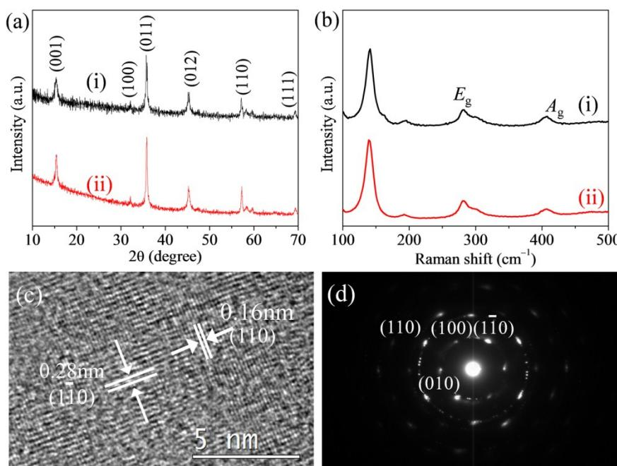
Fig. S1 (a,b) XRD patterns (a) and Raman spectra (b) of the V<sup>2+</sup>-doped VS<sub>2</sub> mesoporous nanosheets before (i) and after (ii) annealing at 350 °C in N<sub>2</sub> atmosphere, showing outstanding thermal stability. (c,d) HRTEM image (c) and SAED pattern (d) of the annealed VS<sub>2</sub> nanosheets.
