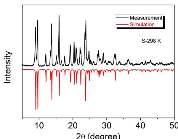
Fig. S2 Pattern of powder X-ray diffraction of *S*-configuration at 298 K, verifying the purity of the bulk phase.
