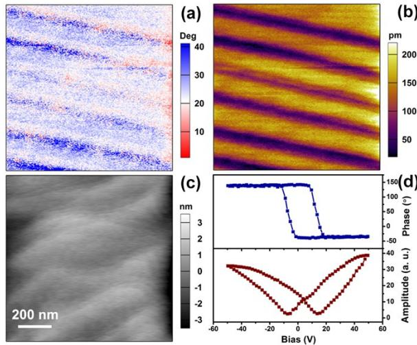
Fig. S6 Domain properties of the thin film of *R*-configuration. Vertical phase (a) and amplitude images (b) and topographic images (c) for the thin film. (d) Phase and amplitude signals as functions of the tip voltage for a selected point, showing local PFM hysteresis loops.
