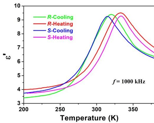
Fig. S4 Temperature-dependent dielectric real part  $\epsilon'$  under 1000 kHz in a heating and cooling cycle with the same heating/cooling rate of 15 K min⁻¹ in terms of polycrystalline samples for *R*- and *S*-configuration.
