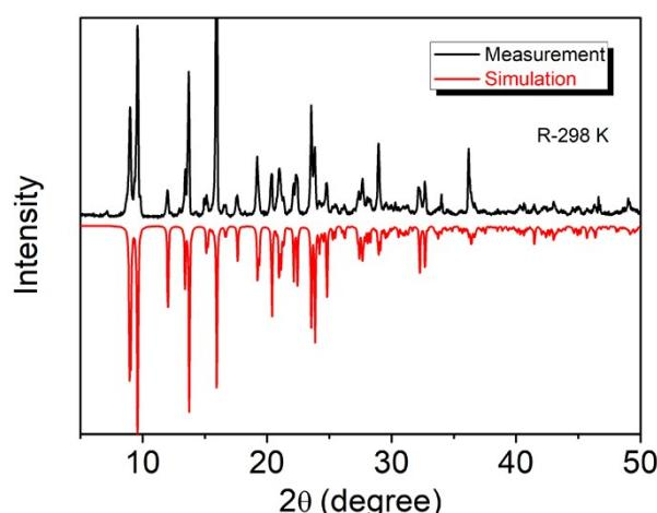
Fig. S1 Pattern of powder X-ray diffraction of *R*-configuration at 298 K, verifying the purity of the bulk phase.
