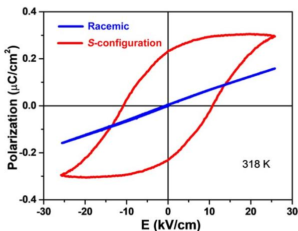
Fig. S5 Comparison of ferroelectric P–E loop of *S*-configuration and racemate at 318 K.
