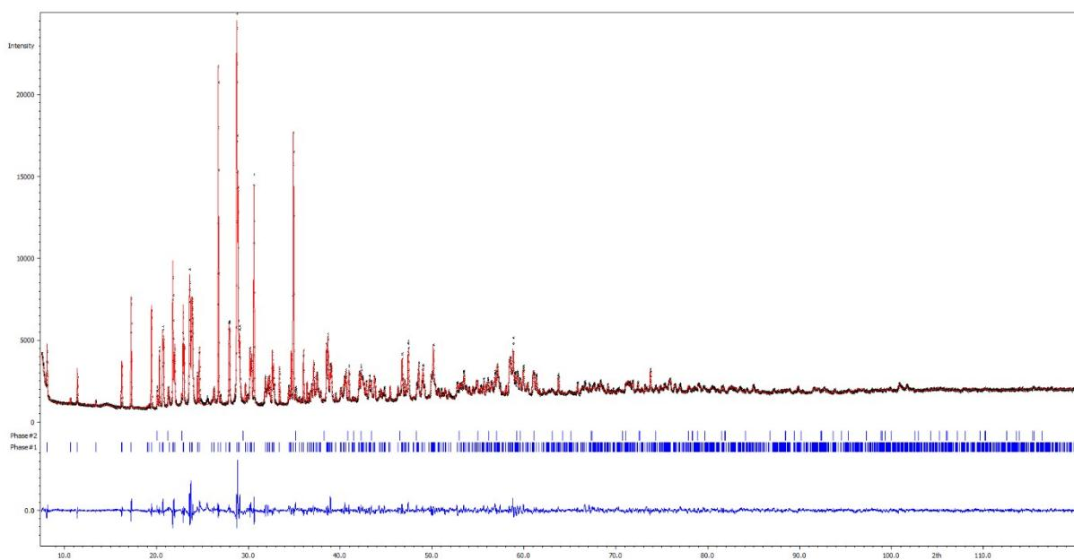
*Figure s2.* PXRD diagram of DFZ-64C-HT at 570°C (Cu-K $\alpha$ 1 radiation; 1.5406 $\text{\AA}$ ) with observed (dots), calculated (solid line), Bragg reflections (ticks), and difference profiles (bottom line) obtained after Rietveld refinements
