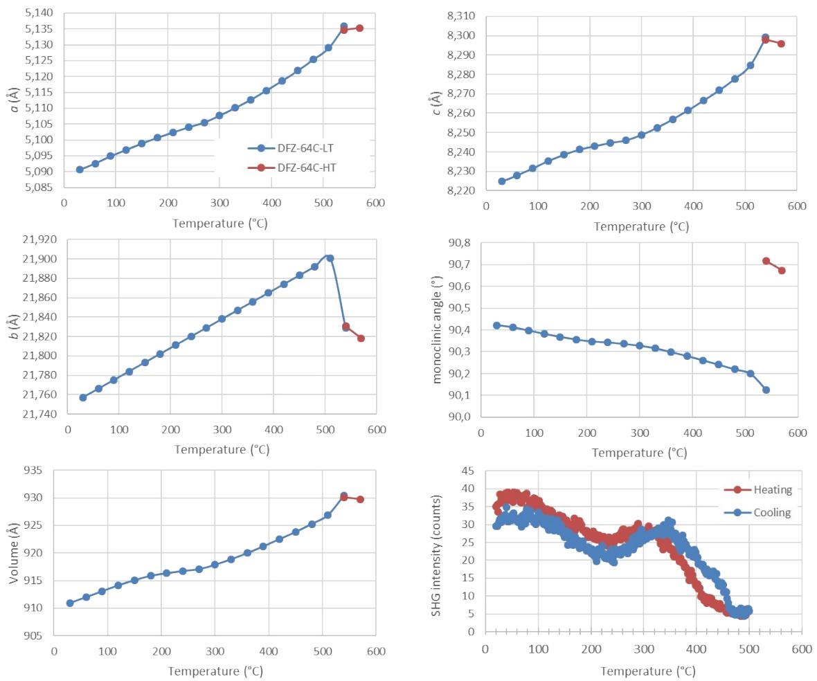
*Figure s1. The variation of the unit-cell parameters and evolution of SHG intensity with the temperature of sample DFZ-64C*
