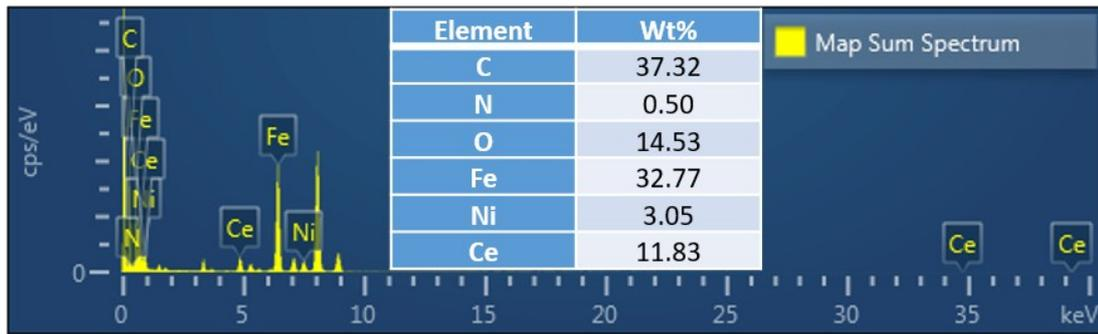
**Fig. S2** The EDS spectrum of the prepared  $\text{Fe}_x\text{Ni}_y/\text{CeO}_2/\text{NC}$ .
