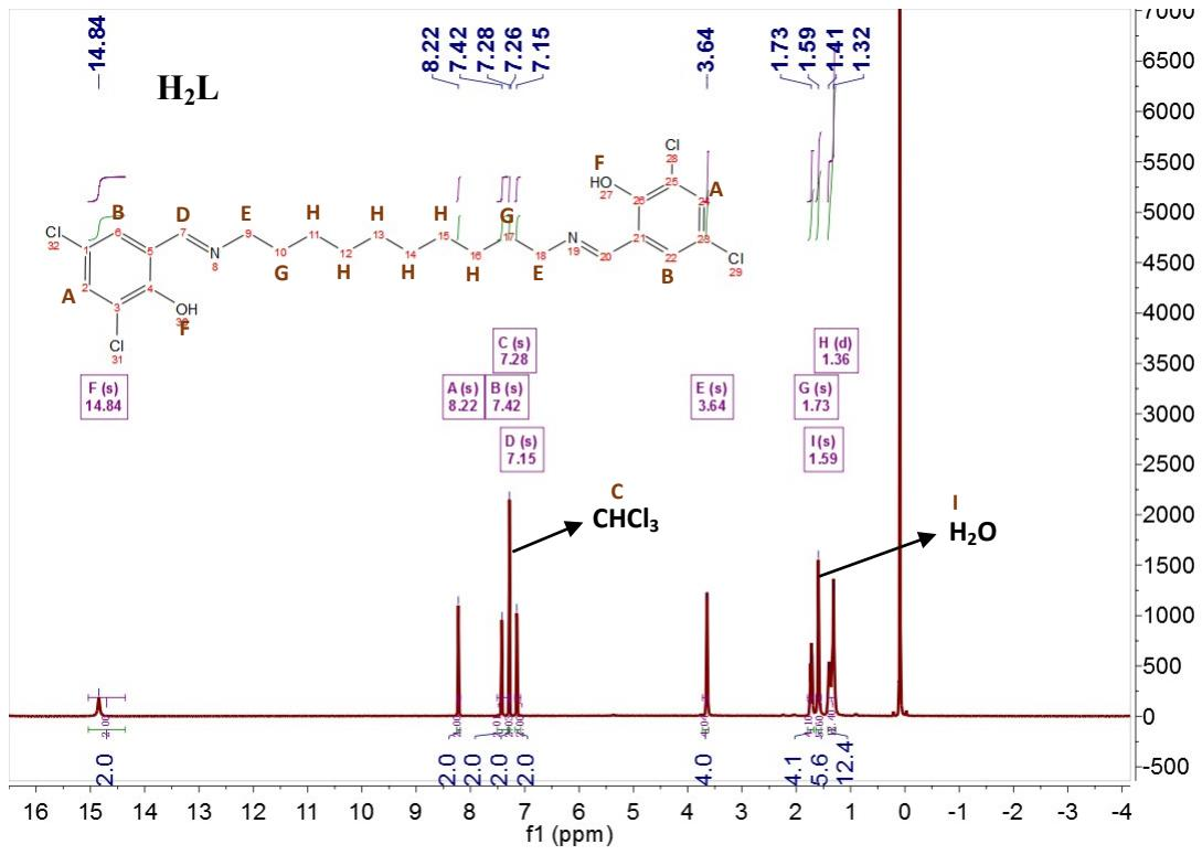
**Figure S1.**  $^1\text{H}$  NMR spectrum of  $\text{H}_2\text{L}$  in  $\text{CDCl}_3$  at room temperature (with assignment of protons from “A” to “I”).
