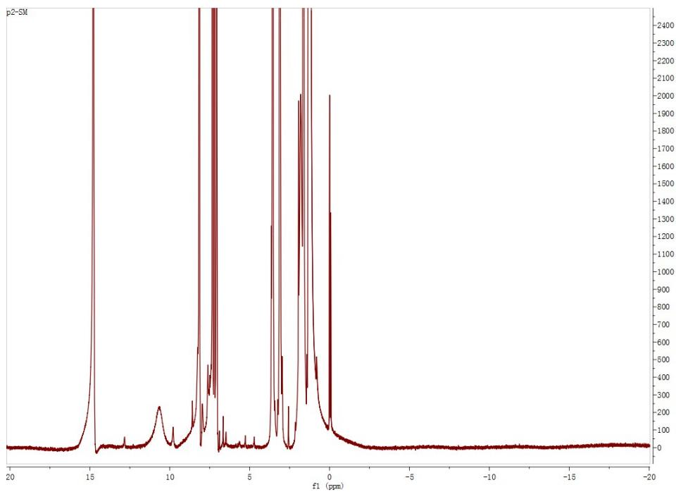
**Figure S5.**  $^1\text{H}$  NMR spectra of **1** in *d*-DMF at room temperature.
