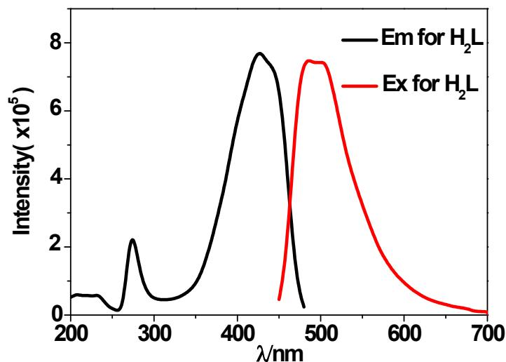
**Figure S6.** The excitation and emission spectra of the free H<sub>2</sub>L in DMF at room temperature. ( $\lambda_{\text{ex}} = 420 \text{ nm}$ ,  $\lambda_{\text{em}} = 500 \text{ nm}$ )
