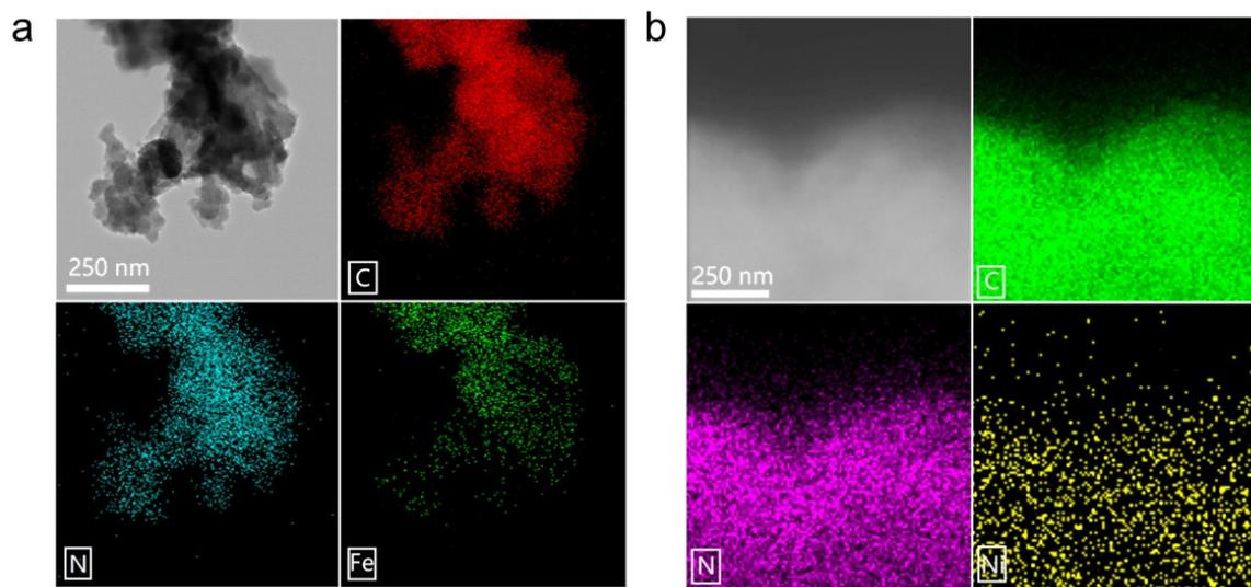
**Fig. S8** The STEM and elemental-mapping images of (a) FePc-CP and (b) NiPc-CP.
