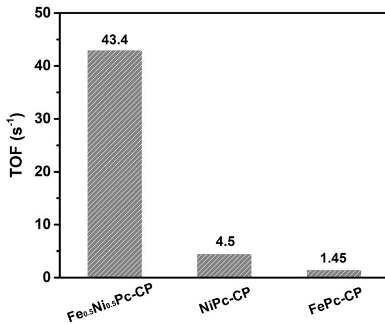
**Fig. S10** Turnover frequency (TOF) of FePc-CP, FePc-CP, and Fe<sub>0.5</sub>Ni<sub>0.5</sub>Pc-CP at the overpotential of 317 mV.
