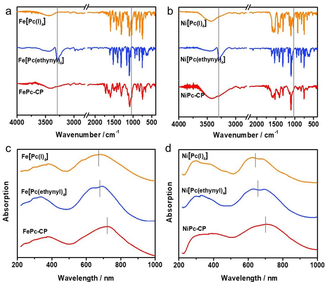
**Fig. S5** (a) FT-IR and (c) solid-state UV-vis diffuse reflectance spectra of FePc-CP and corresponding phthalocyanine monomers. (b) FT-IR and (d) Solid-state UV-vis diffuse reflectance spectra of NiPc-CP and corresponding phthalocyanine monomers.
