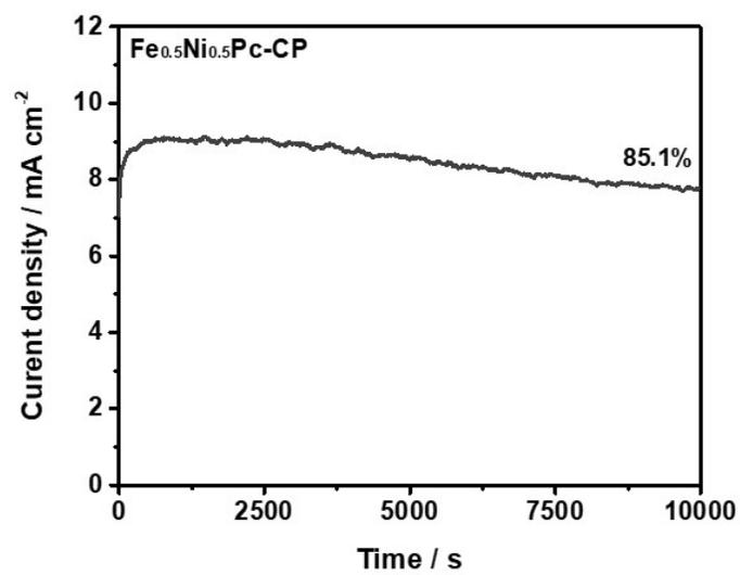
**Fig. S11** Amperometric *i*-*t* curve of Fe<sub>0.5</sub>Ni<sub>0.5</sub>Pc-CP-modified electrode tested with the rotation speed of 1600 rpm in 1.0 M KOH solution.
