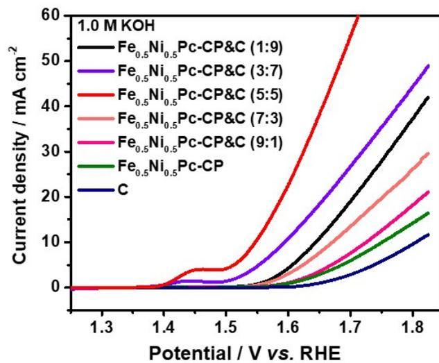
**Fig. S9** LSV curves of pure XC-72 and Fe<sub>0.5</sub>Ni<sub>0.5</sub>Pc-CP mixture with different contents measured at the scan rate of 10 mV s<sup>-1</sup> with the rotation speed of 1600 rpm in 1.0 M KOH solution.
