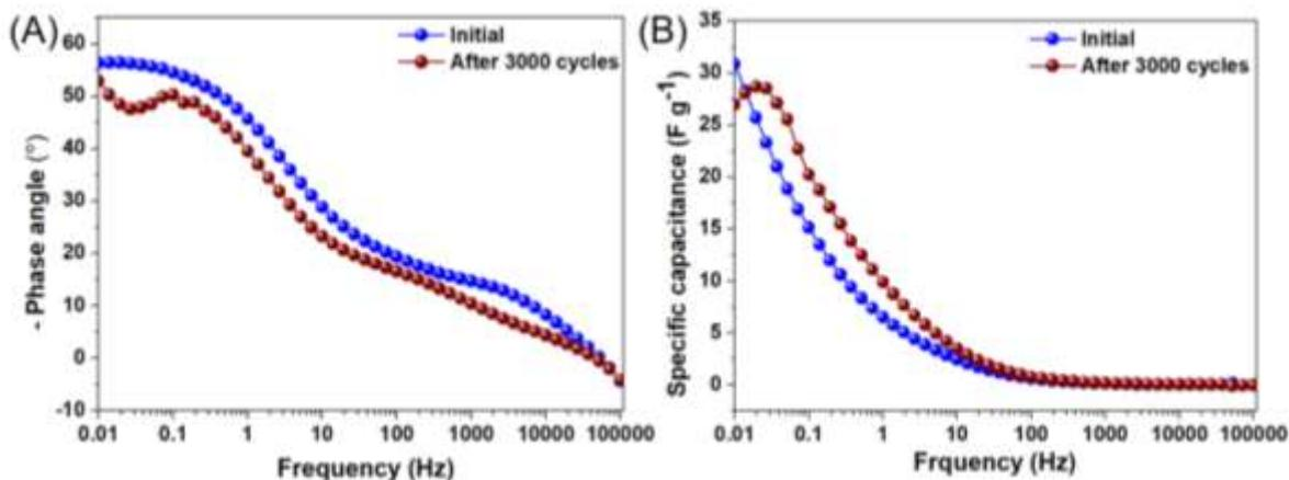
**Figure S10.** (A) Bode phase angle plot initial and after 3000 cycles of CuFeS<sub>2</sub>||CuFeS<sub>2</sub> SSD, and (B) Plot of variation of specific capacitance of CuFeS<sub>2</sub>||CuFeS<sub>2</sub> SSD with respect to frequency at initial and after 3000 cycles.
