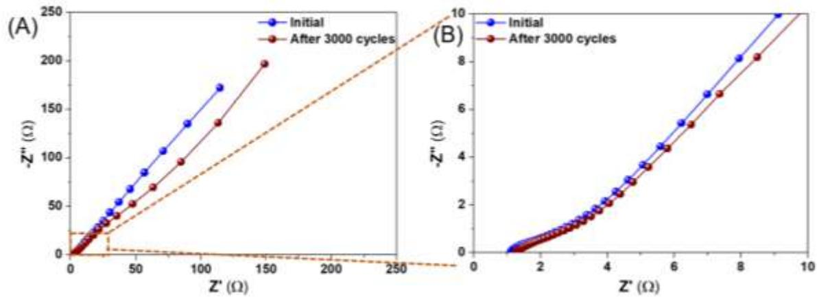
**Figure S9.** (A) Nyquist plot of CuFeS<sub>2</sub>||CuFeS<sub>2</sub> SSD measured during initial and after 3000 cycles, and (B) enlarged view of Nyquist plot of CuFeS<sub>2</sub>||CuFeS<sub>2</sub> SSD.
