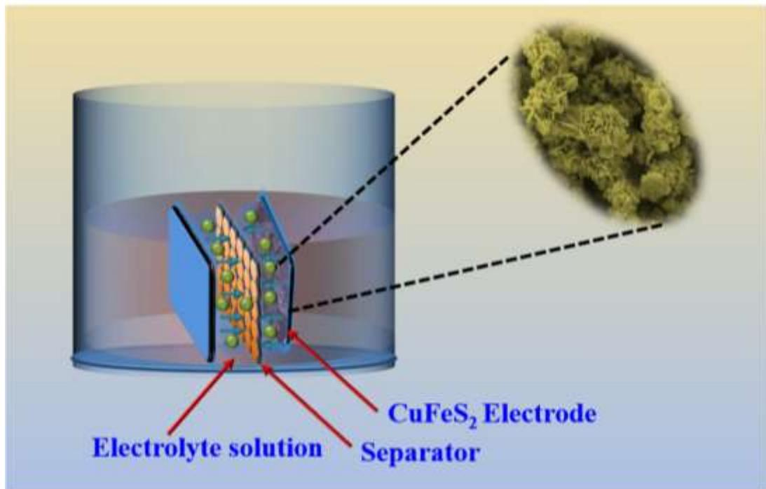
**Figure S7.** Schematic illustration of the fabrication of CuFeS<sub>2</sub>||CuFeS<sub>2</sub> SSD.
