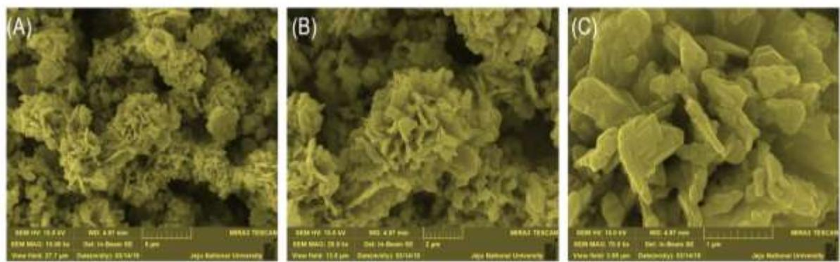
**Figure S1.** Field emission-scanning electron (FE-SEM) micrographs of as prepared CuFeS<sub>2</sub> (A-C) at different magnification (10.0 kx, 20.0 kx, and 70.0 kx).
