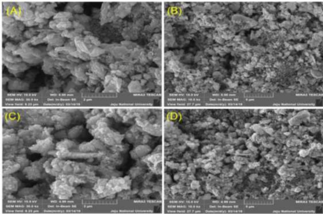
Figure S11. FE-SEM micrograph of as fabricated CuFeS<sub>2</sub> electrode (A and B) before electrochemical test, and (C and D) after cyclic stability test.
