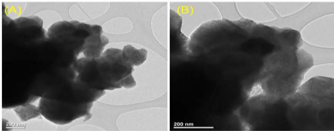
**Figure S3.** The highly magnified HR-TEM image to confirming the presence numerous hierarchically porous and interconnected CuFeS<sub>2</sub> platelet network.
