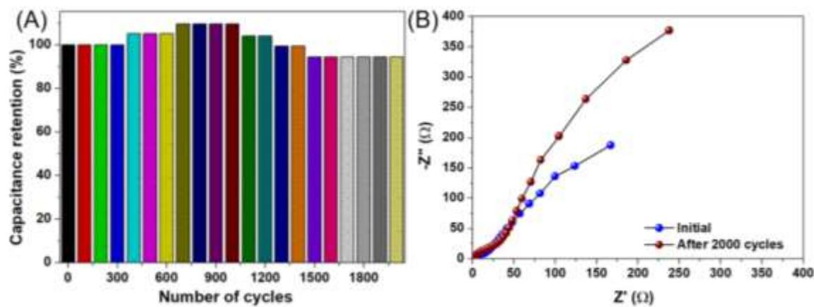
**Figure S6.** (A) Cyclic stability performance of CuFeS<sub>2</sub> electrode over 2000 cycles, and (B) Nyquist plot of CuFeS<sub>2</sub> electrode measured during initial and after the 2000 cycle.
