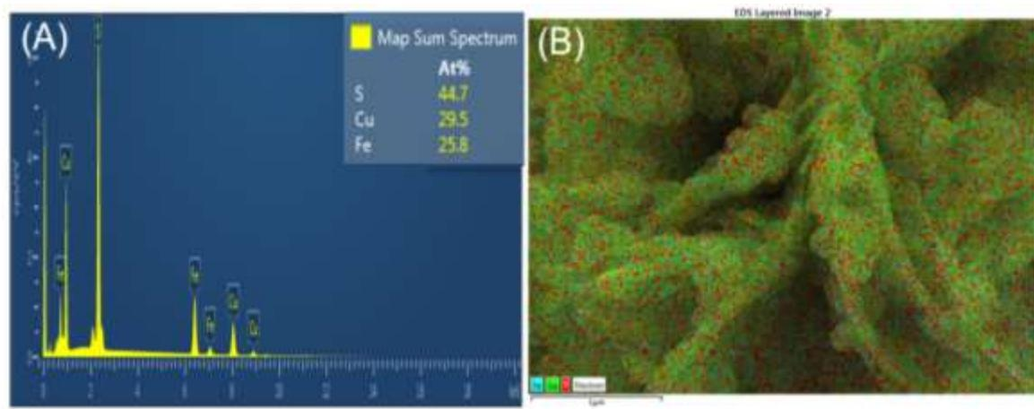
**Figure S2.** (A) EDX spectrum of as prepared CuFeS<sub>2</sub>, and (B) FE-SEM micrographs for elemental mapping of CuFeS<sub>2</sub>.
