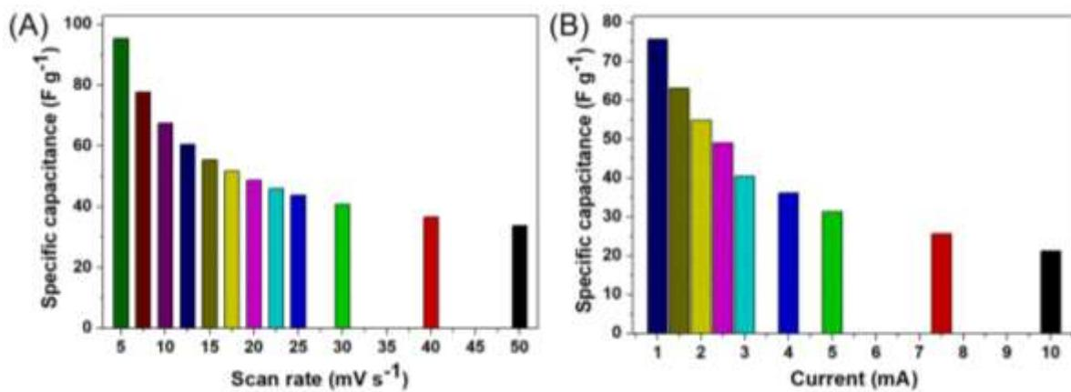
**Figure S4.** (A) Effect of specific capacitance of CuFeS<sub>2</sub> electrode with respect to scan rate, and (B) Effect of specific capacitance of CuFeS<sub>2</sub> electrode with respect to current.
