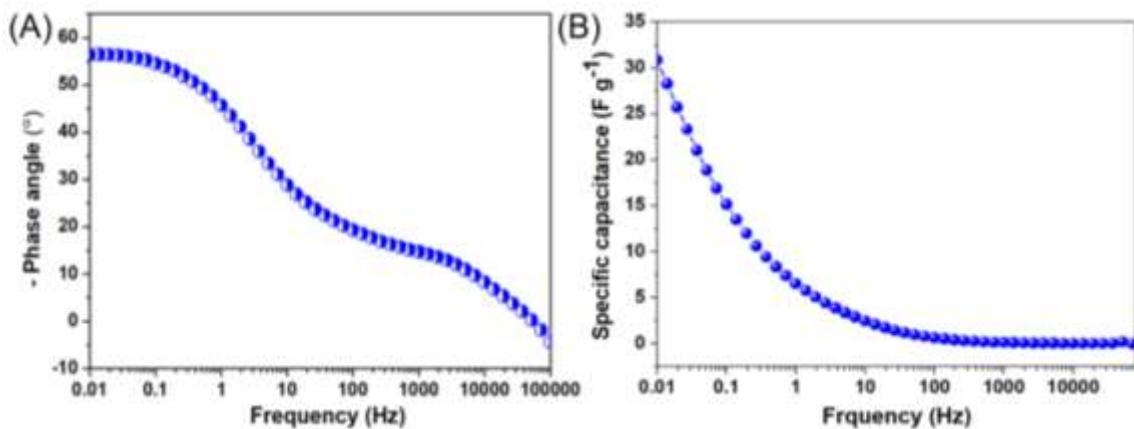
**Figure S8.** EIS analysis of CuFeS<sub>2</sub>||CuFeS<sub>2</sub> SSD (A) Bode phase angle plot, and (B) Plot of variation of specific capacitance of CuFeS<sub>2</sub>||CuFeS<sub>2</sub> SSD with respect to frequency.
