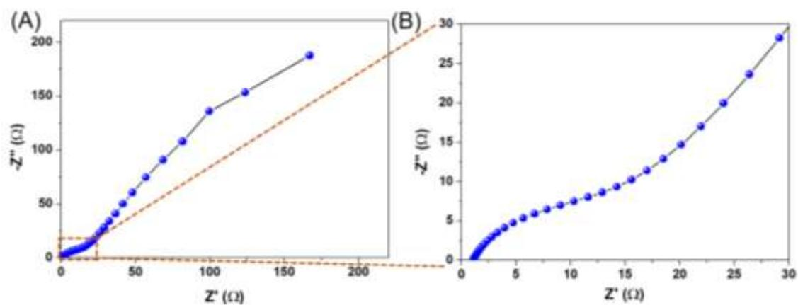
**Figure S5.** (A) Nyquist plot of CuFeS<sub>2</sub> electrode, and (B) enlarged view of the Nyquist plot of CuFeS<sub>2</sub> electrode.
