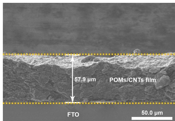
**Fig. S10.** The cross sectional view of the Co<sub>4</sub>PW<sub>9</sub>/CNTs CE.
