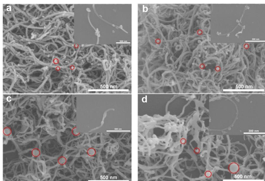
**Fig. S11.** The SEM images of (a) PW<sub>12</sub>/CNTs, (b) PMo<sub>12</sub>/CNTs, (c) P<sub>2</sub>W<sub>18</sub>/CNTs and (d) P<sub>2</sub>Mo<sub>18</sub>/CNTs nanocomposites.
