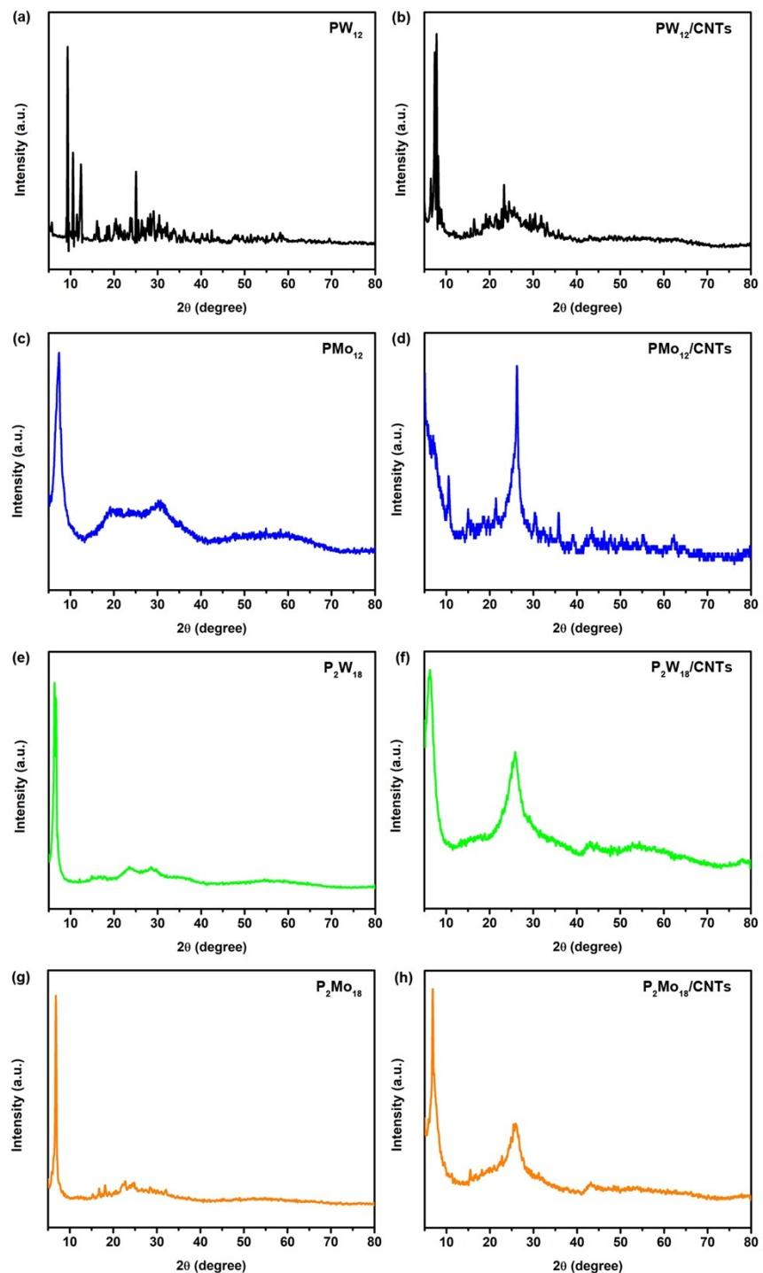
**Fig. S2.** The PXRD patterns of (a, c, e, g) POMs salts; (b, d, f, h) POMs/CNTs nanocomposites employed as the CEs.
