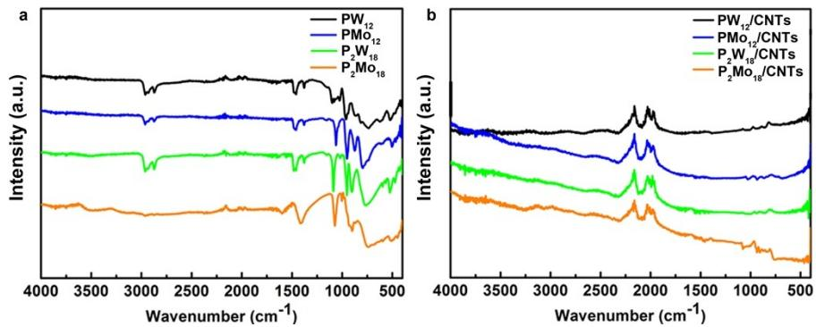
**Fig. S1.** IR spectra of POMs salts, POMs/CNTs nanocomposites employed as the CEs.
