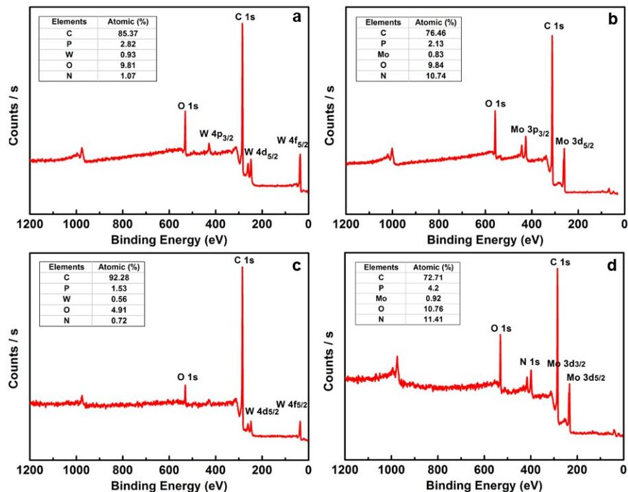
**Fig. S4.** The full XPS spectra of (a) PW<sub>12</sub>/CNTs, (b) PMo<sub>12</sub>/CNTs, (c) P<sub>2</sub>W<sub>18</sub>/CNTs and (d) P<sub>2</sub>Mo<sub>18</sub>/CNTs nanocomposites.
