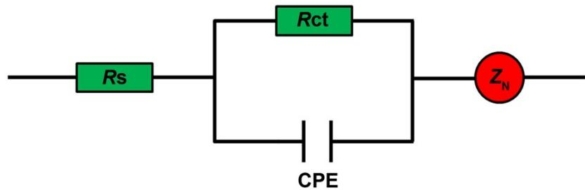
**Fig. S13.** The equivalent circuit for EIS analysis;  $R_s$  is the series resistance, CPE represents the electrochemistry double-layer capacitance, the charge transfer resistance related to the IRR process is  $R_{ct}$ .
