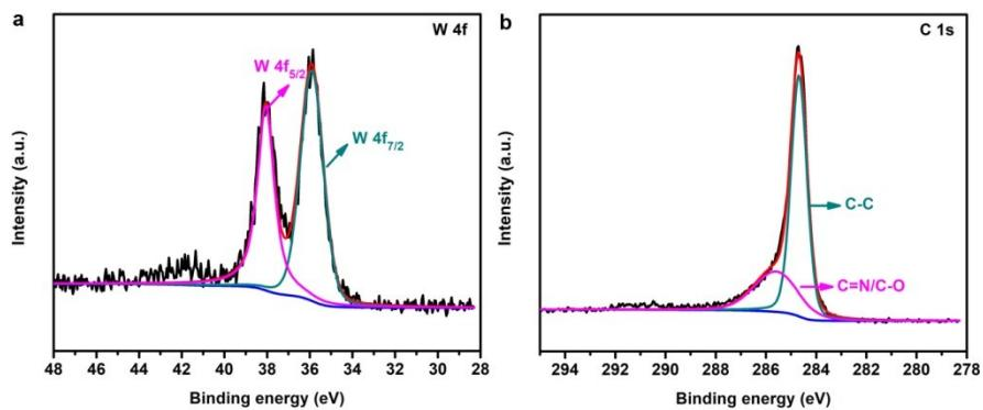
**Fig. S7.** High-resolution XPS spectra of (a) W and (b) C in P<sub>2</sub>W<sub>18</sub>/CNTs nanocomposite.
