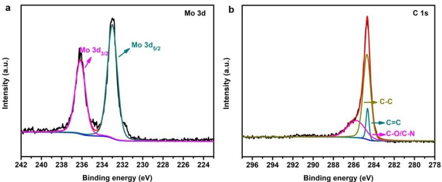
**Fig. S8.** High-resolution XPS spectra of (a) Mo and (b) C in P<sub>2</sub>Mo<sub>18</sub>/CNTs nanocomposite.
