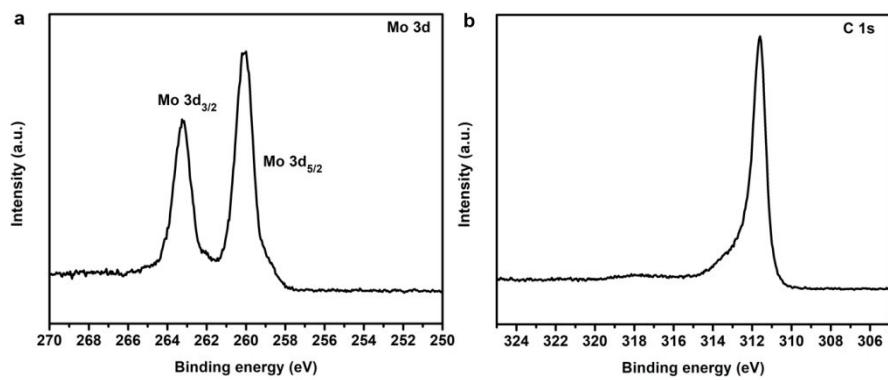
**Fig. S6.** High-resolution XPS spectra of (a) Mo and (b) C in PMo<sub>12</sub>/CNTs nanocomposite.
