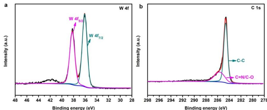
**Fig. S5.** High-resolution XPS spectra of (a) W and (b) C in PW<sub>12</sub>/CNTs nanocomposite.
