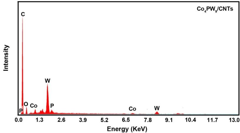
**Fig. S3.** The EDX result of  $\text{Co}_4\text{PW}_9/\text{CNTs}$  nanocomposites.
