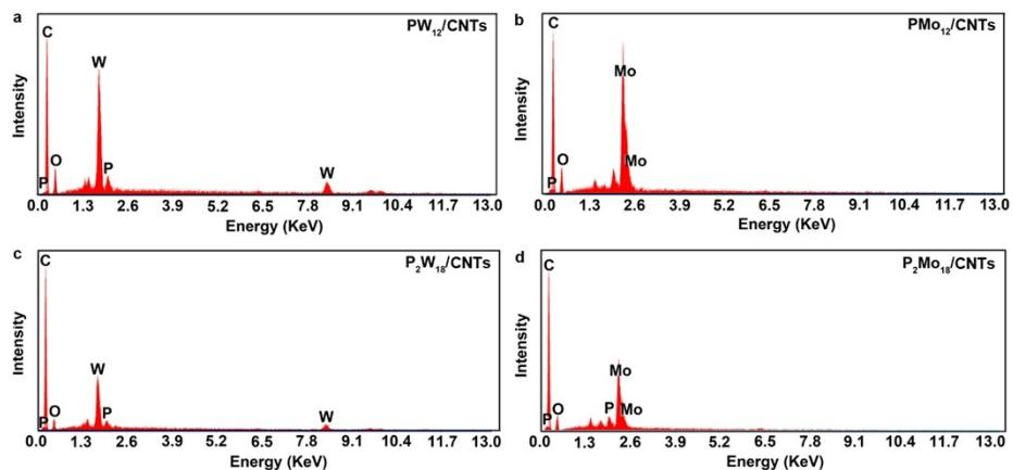
**Fig. S9.** The EDX results of (a) PW<sub>12</sub>/CNTs, (b) PMo<sub>12</sub>/CNTs, (c) P<sub>2</sub>W<sub>18</sub>/CNTs and (d) P<sub>2</sub>Mo<sub>18</sub>/CNTs nanocomposites.
