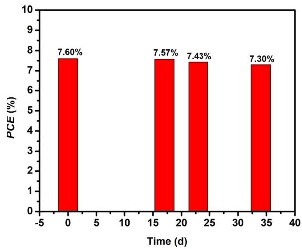
**Fig. S14.** Long-term stability of a DSSC based on  $\text{Co}_4\text{PW}_9/\text{CNTs}$  CE.
