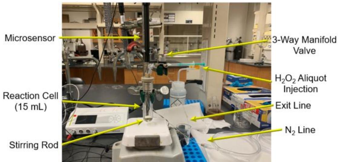
**Figure S2.** O<sub>2</sub> measurement setup using an O<sub>2</sub> microsensor (Unisense) for quantifying O<sub>2</sub> produced by H<sub>2</sub>O<sub>2</sub> disproportionation.
