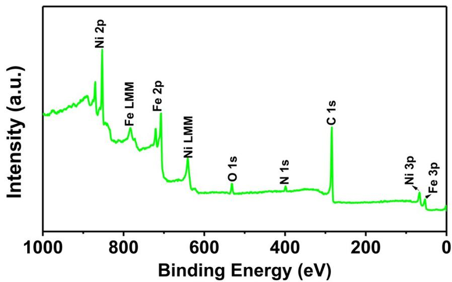
Fig. S5. Survey XPS spectrum of sample S2.
