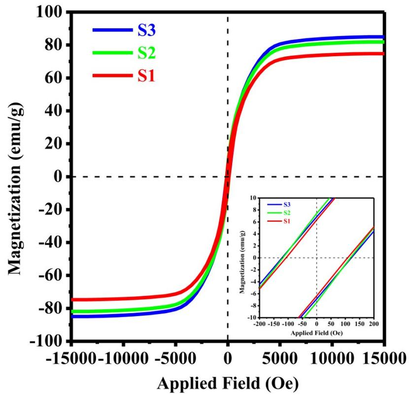
Fig. S4. Magnetization hysteresis loops of the as-prepared samples S1 (red), S2 (green) and S3 (blue).
