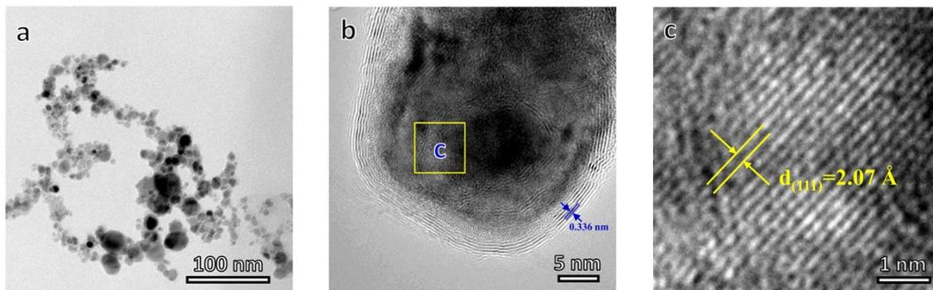
Fig. S2. TEM (a) and HRTEM (b and c) images of the prepared NiFe@C nanoparticle (S0).
