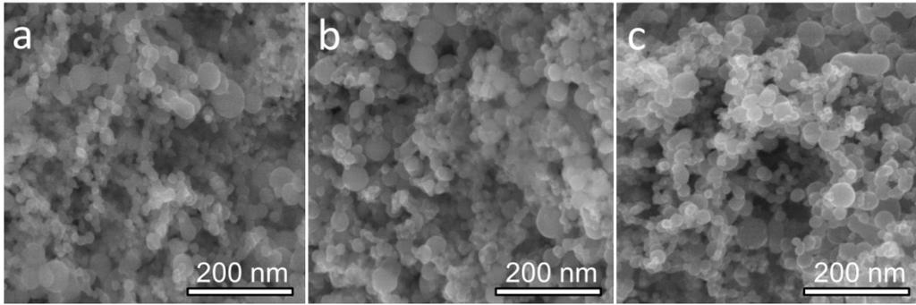
Fig. S1. SEM images of the as-made NiFe@NC nanoparticles, (a) S1, (b) S2 and (c) S3. From these images, it can be seen that all of the three samples are composed of irregular spherical particles less than 100 nm in size.
