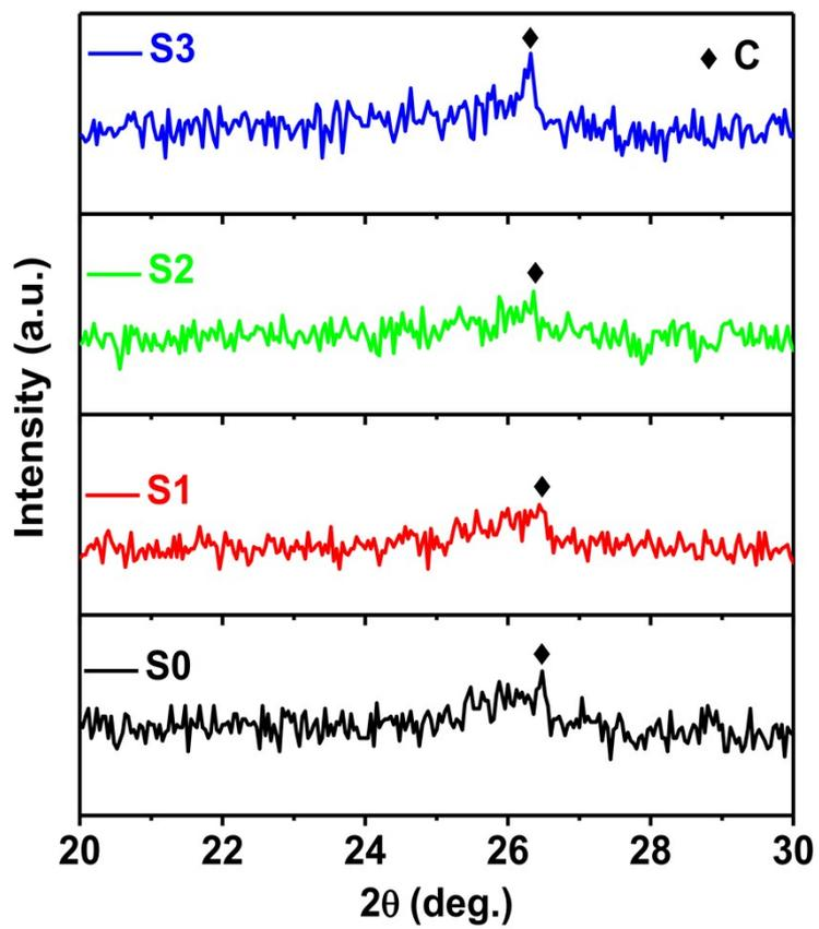
Fig. S3. Enlarged XRD patterns from  $20^\circ$  to  $30^\circ$  of the as-prepared samples S0 (black), S1 (red), S2 (green) and S3 (blue).
