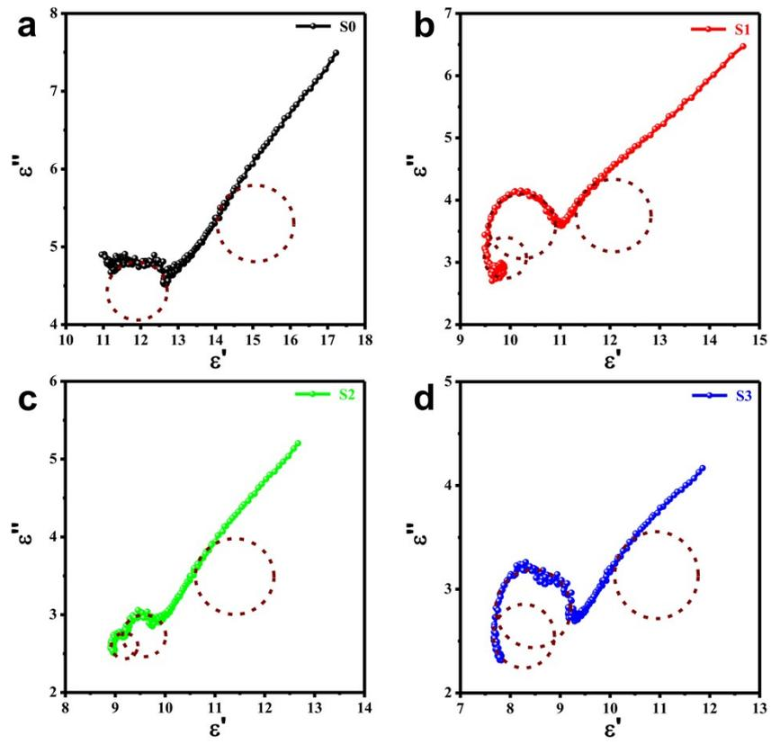
Fig. S6. The Cole-Cole circles of samples S0 (a), S1 (b), S2 (c) and S3 (d).
