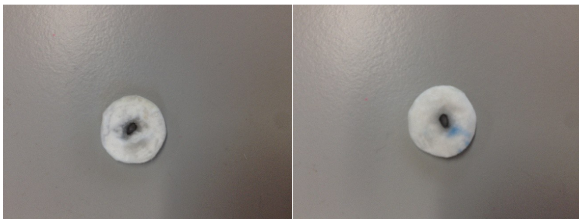
Figure S1: Photographs of the separators of a Mg-metal symmetrical cell with TCE electrolyte after the short-circuit in the polarisation test. A clear grey metallic spot can be observed at both sides of the separator.
