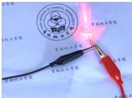
**Figure S6.** The photograph of an LED is powered by the two ASCs in series.
