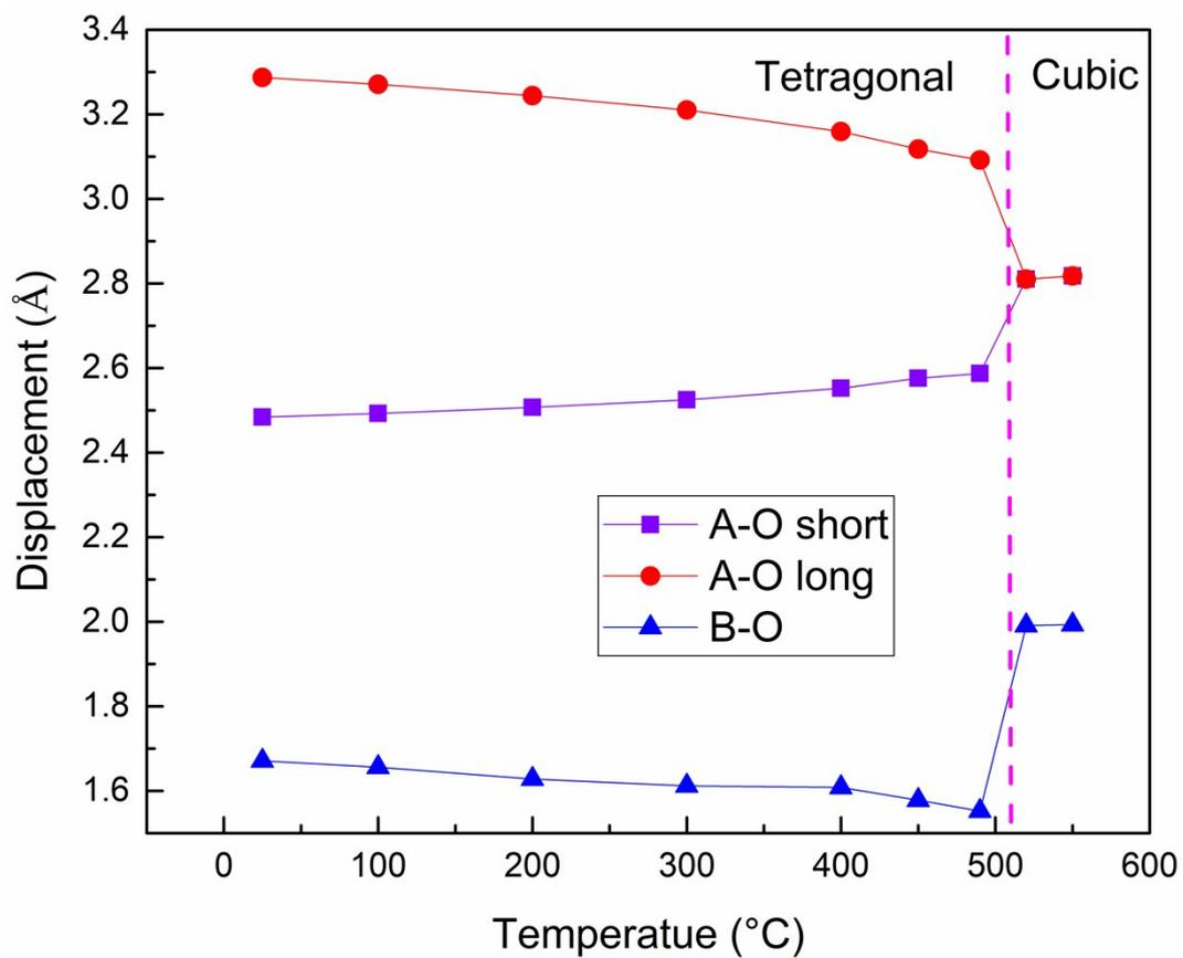
**Figure S4** The temperature dependent of the displacement of A-site to O2 short, A-site to O2 long and B-site to O1 in  $0.85\text{PbTiO}_3\text{-}0.15\text{Bi}(\text{Zn}_{2/3}\text{Ta}_{1/3})\text{O}_3$ . Because of charge disproportionation existed, the bond length changes with the increasing of temperature.
