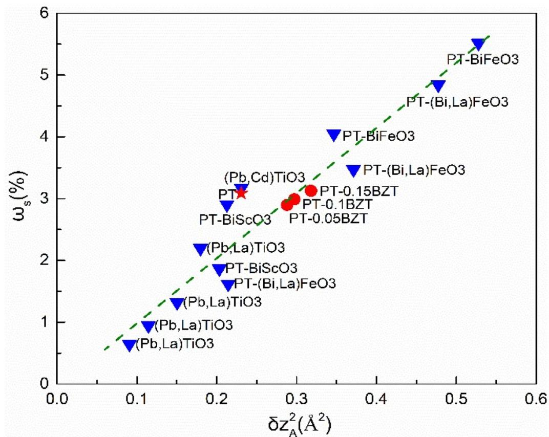
**Figure S3** The correlation between the spontaneous volume ferroelectrostriction ( $\omega_s$ ) and square of  $P_S$  displacement ( $\delta z_A^2$ ) for PT-based tetragonal NTE ferroelectrics according to SVFS theory.<sup>1</sup>
