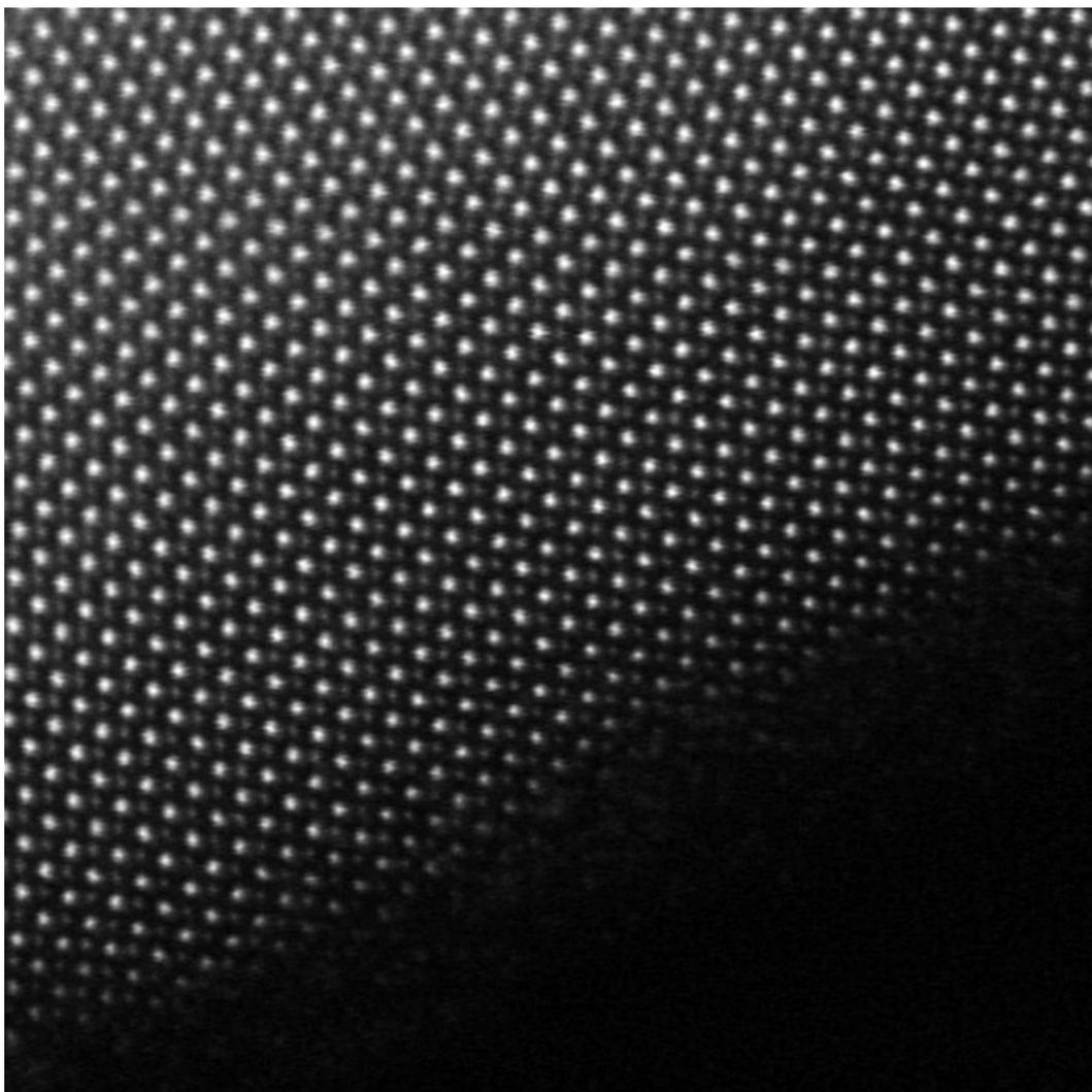
**Figure S5** The STEM image of  $0.85\text{PbTiO}_3\text{-}0.15\text{Bi}(\text{Zn}_{2/3}\text{Ta}_{1/3})\text{O}_3$ .
