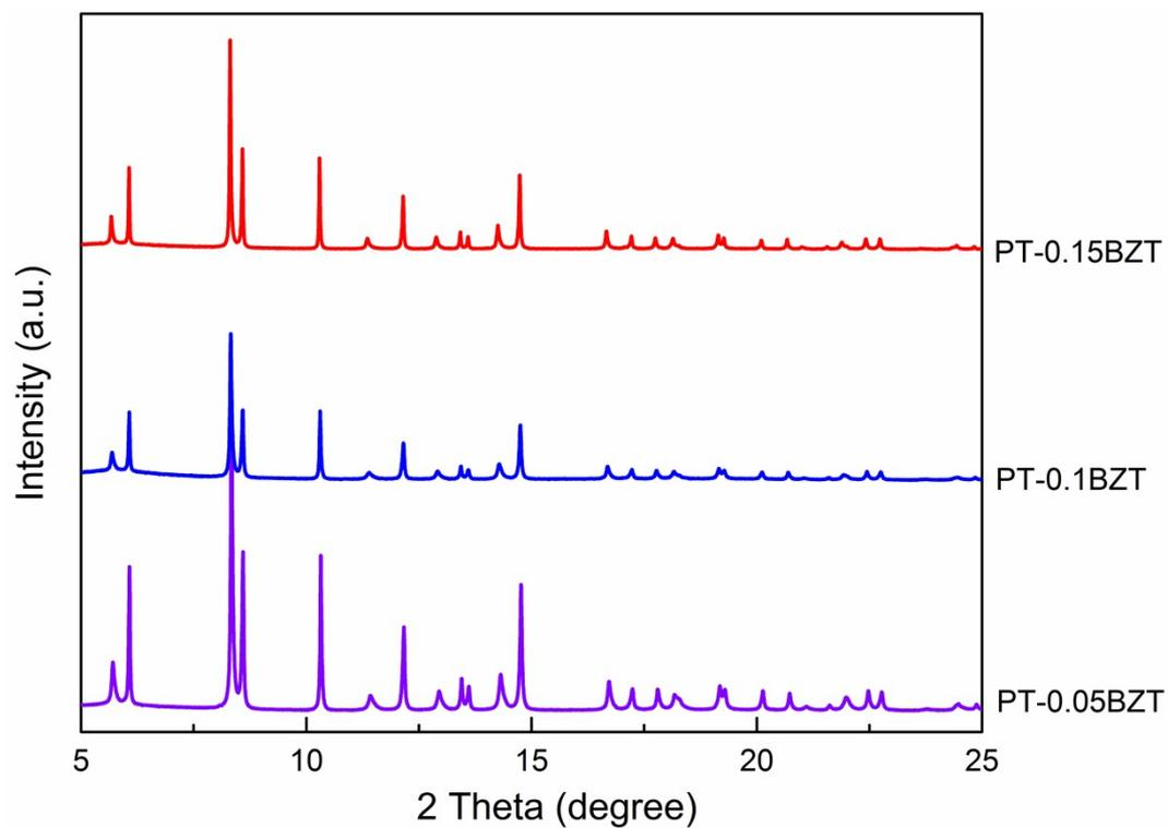
**Figure S1** The synchrotron XRD patterns of  $(1-x)\text{PbTiO}_3-x\text{Bi}(\text{Zn}_{2/3}\text{Ta}_{1/3})\text{O}_3$  ( $x = 0\sim 0.2$ ) at room temperature.
