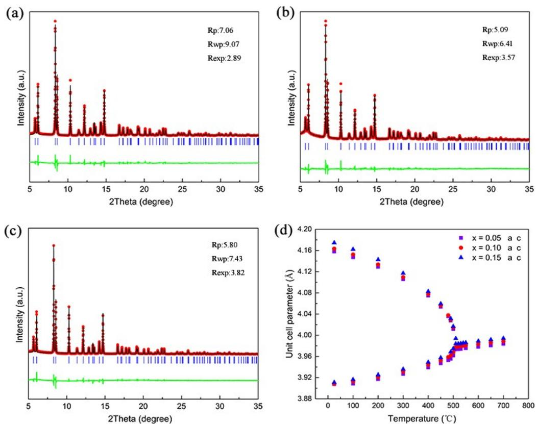
**Figure S2** Rietveld refinement of the synchrotron XRD patterns of  $(1-x)\text{PbTiO}_3-x\text{Bi}(\text{Zn}_{2/3}\text{Ta}_{1/3})\text{O}_3$  ((a):  $x = 0.05$ ; (b):  $x = 0.10$ ; (c):  $x = 0.15$ ) at room temperature.
